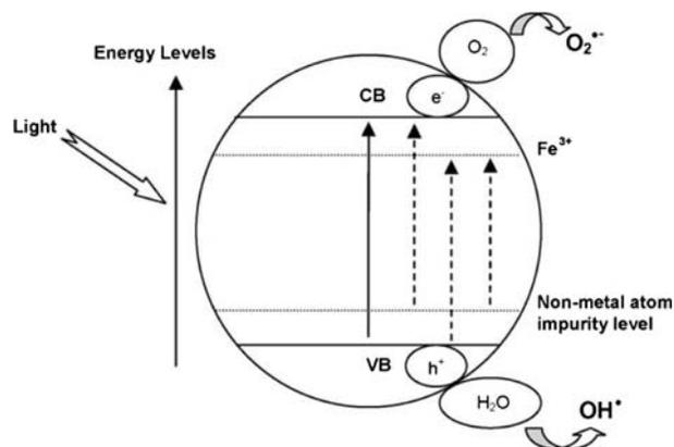
Fig. 6. Schematic diagram of doped- $TiO_2$  and initial redox process after activation by light [6,13].
