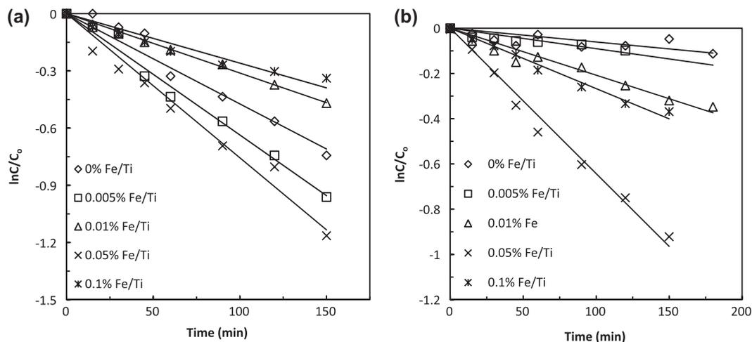
Fig. 4. Pseudo-first-order kinetics of phenol degradation using different Fe/Ti weight ratios under (a) solar radiation and (b) pure visible light.
