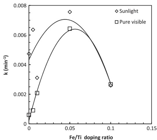
Fig. 5. Change in pseudo-first order rate constant of phenol degradation using different Fe/Ti doping ratios under sunlight and pure visible light.
