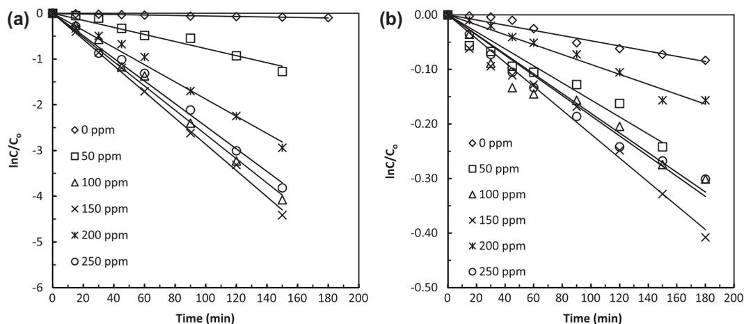
Fig. 7. Effect of catalyst concentration on phenol degradation using 0.05% Fe/Ti doping ratio under (a) sunlight and (b) pure visible irradiation.
