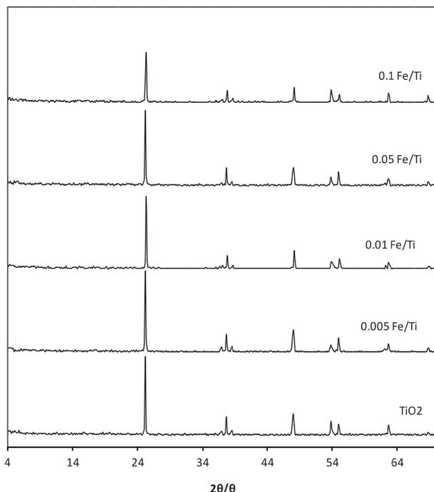
Fig. 2. XRD patterns of prepared photocatalysts of different Fe/Ti atomic ratios.
