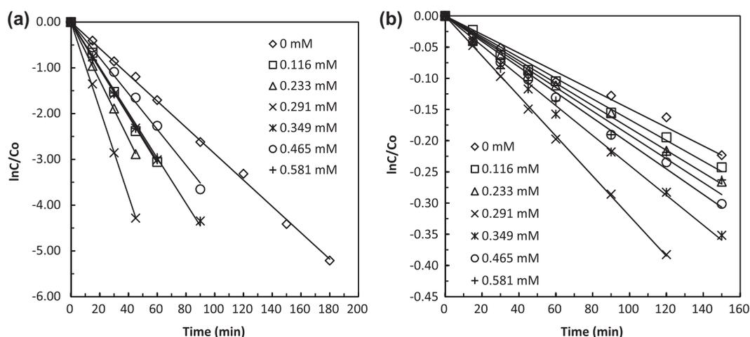
Fig. 8. Effect of  $\text{H}_2\text{O}_2$  dose on pseudo-first order rate constant of phenol degradation (a) sunlight and (b) pure visible light irradiations using 0.05% Fe/Ti doping ratio.
