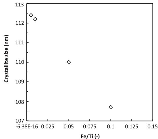
Fig. 3. Effect of Fe/Ti doping ratio on the crystallite size of  $\text{TiO}_2$ .
