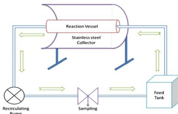
Fig. 1. Schematic diagram of the solar photocatalytic oxidation unit.
