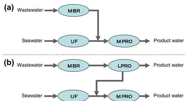
Fig. 1. Flow examples of integrated membrane system of seawater desalination and wastewater reclamation.
