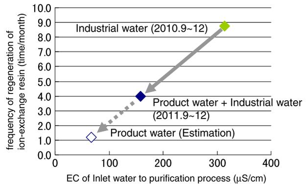
Fig. 7. Relationship between inlet water EC of purification process and monthly frequency of regeneration of ion-exchange resin.
