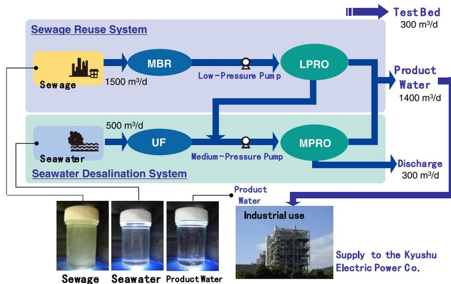
Fig. 2. The schematic flow of “demo plant” built in Kitakyushu, Japan.
