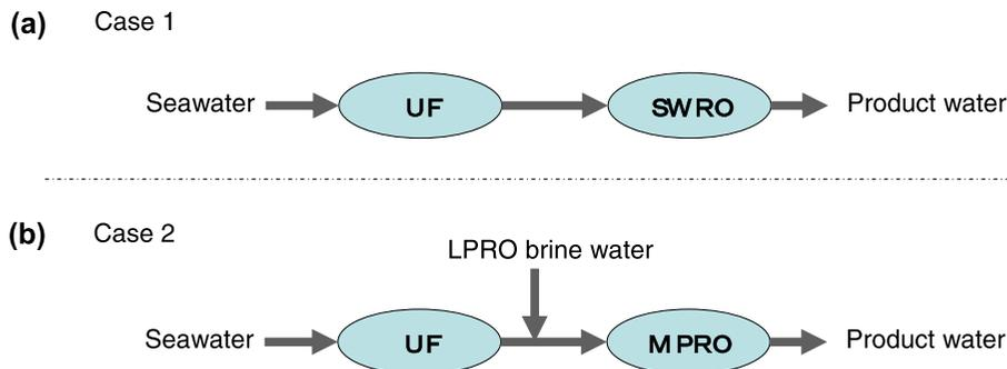
Fig. 8. Basic flow of case study to estimate energy saving; (a) Case 1: the comparative controlled flow, (b) Case 2: the integrated system of seawater desalination and sewage reclamation.
