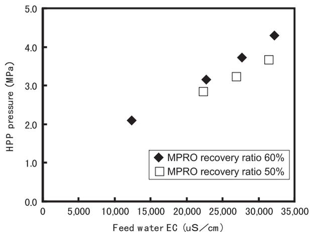
Fig. 4. Relationship between HPP pressure and feed water EC.
