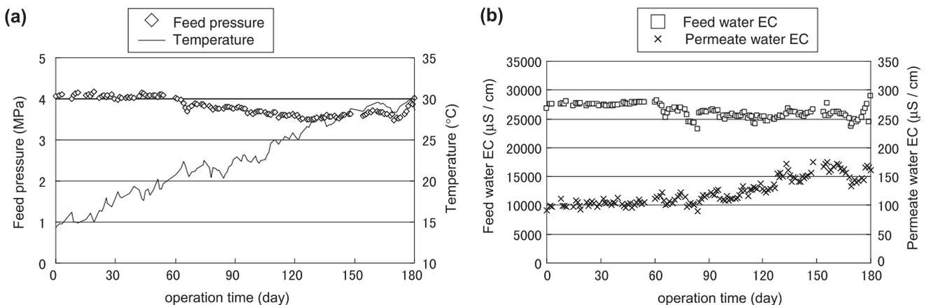
Fig. 5. Time course of feed pressure and water temperature (a), feed water EC and permeate water EC (b).
