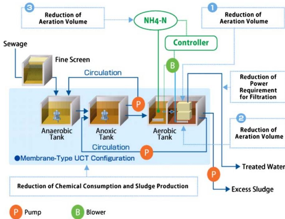
Fig. 3. Basic configuration of MBR and points to realize energy saving.
