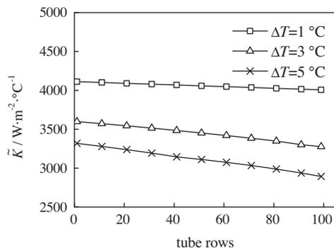
Fig. 9. Result of total temperature difference on bundle-depth effect.
