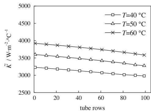
Fig. 7. Result of saturation temperature on bundle-depth effect.
