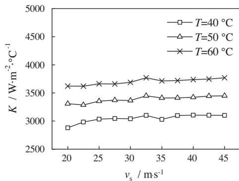
Fig. 5. Effect of steam entrance velocity on overall heat transfer coefficient.
