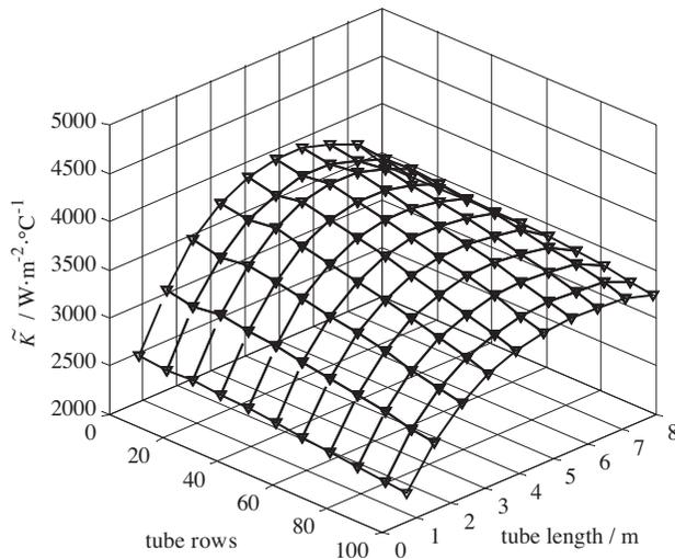
Fig. 10. Space distribution of the  $\tilde{K}$  in the evaporator.
