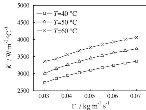
Fig. 3. Effect of spray density and saturation temperature on overall heat transfer coefficient.
