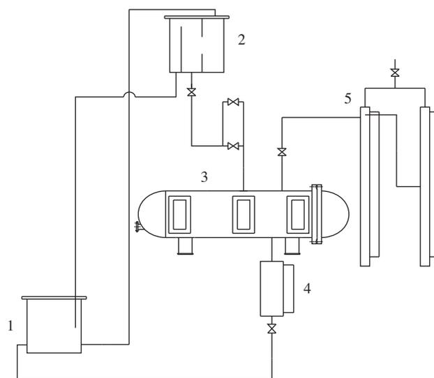
1 heating tank 2 constant pressure liquid feeder 3 evaporator
