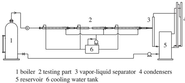
Fig. 2. Schematic diagram of condensation inside a horizontal tube.
