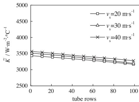
Fig. 8. Result of inlet steam velocity on bundle-depth effect.
