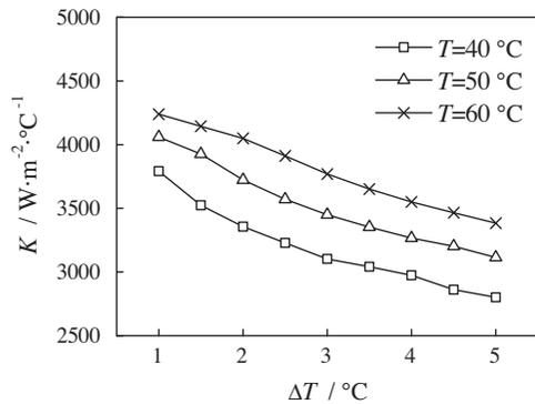
Fig. 4. Effect of total temperature difference on overall heat transfer coefficient.
