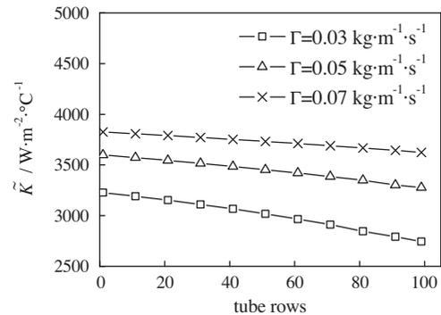
Fig. 6. Result of spray density on bundle-depth effect.
