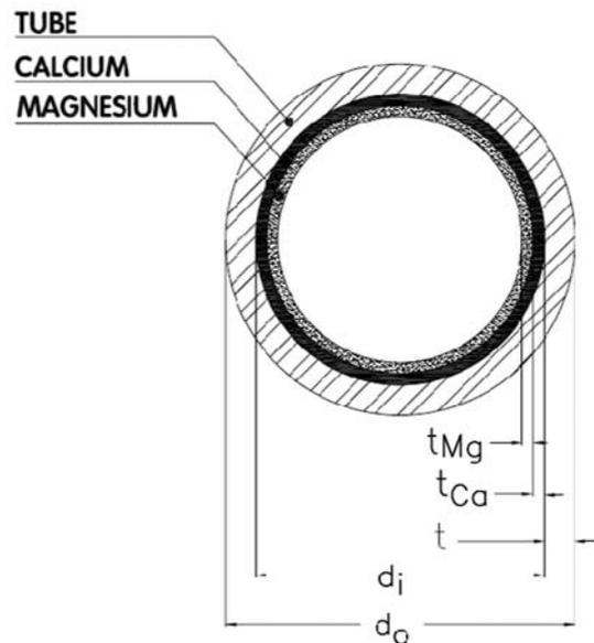
Fig. 10. Schematic diagram inside the scaled tubes.
