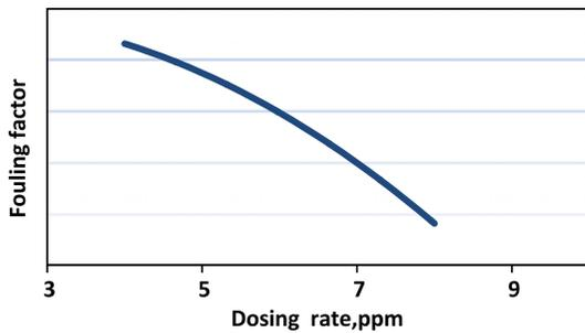
Fig. 11. Fouling factor at 50 g/l salinity without ball cleaning.
