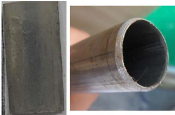
Fig. 5. Coupon and tube samples—without ball cleaning.
