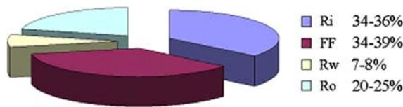
Fig. 2. Heat transfer resistances in MSF condenser.
