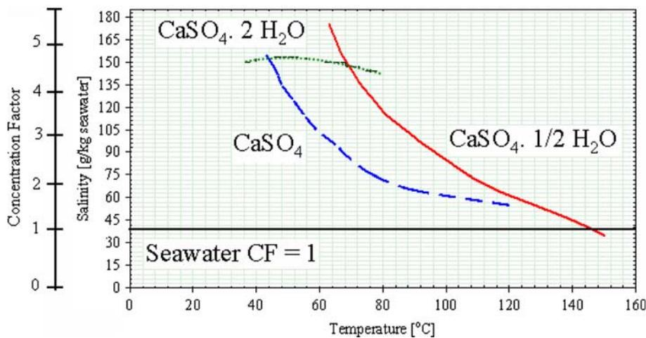
Fig. 3. Phase diagram of  $\text{CaSO}_4$ .
