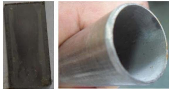
Fig. 6. Coupon and tube samples—with ball cleaning.
