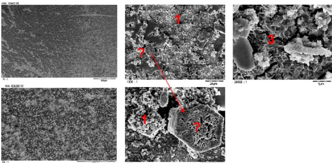
Fig. 7. SEM result at TBT = 120 °C, salinity 60 g/l, and dosing rate = 2.5 ppm.
