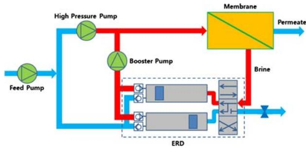
Fig. 2. A conceptual diagram of PEER system.
