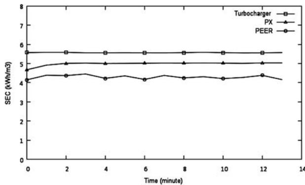
Fig. 6. The SEC of the RO processes by ERD mode in 2 February 2012.
