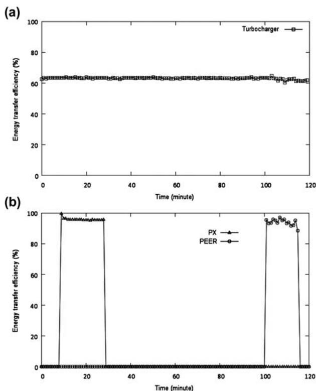
Fig. 4. Comparison of ERD energy transfer efficiency per class of RO in 2 February 2012: (a) ERD operation data of the second RO process and (b) ERD operation data of the first RO process.
