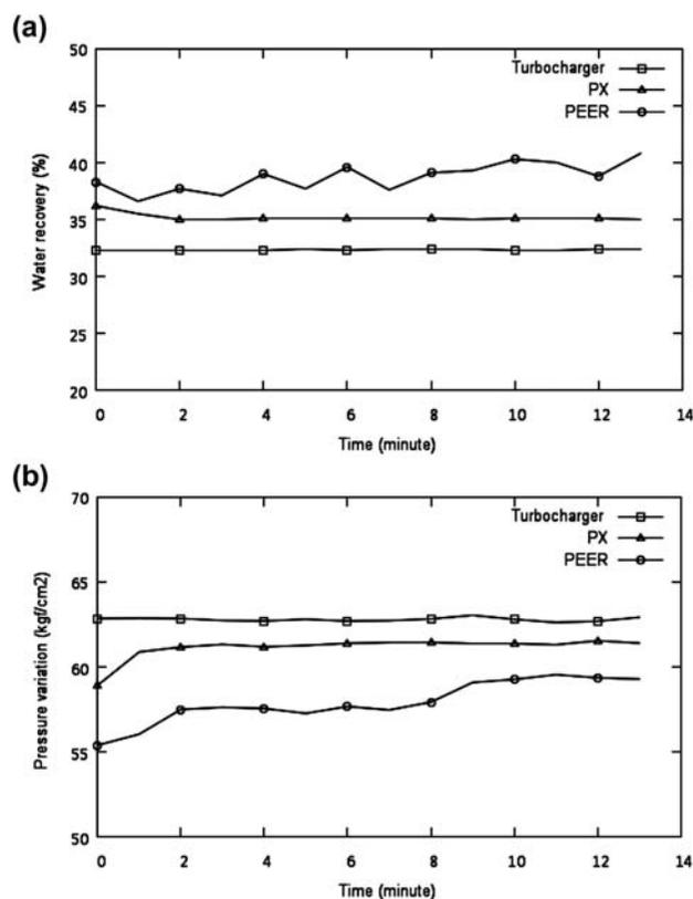
Fig. 5. Effect of the ERD mode on the performances of RO processes in 2 February 2012: (a) water recovery variations and (b) pressure variations between raw water and pressurized feed water.
