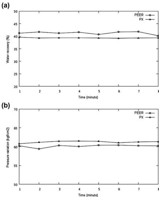
Fig. 7. Comparisons of operational performances between two isobaric systems in 5 March 2012: (a) water recovery variations and (b) pressure variations between raw water and pressurized feed water.
