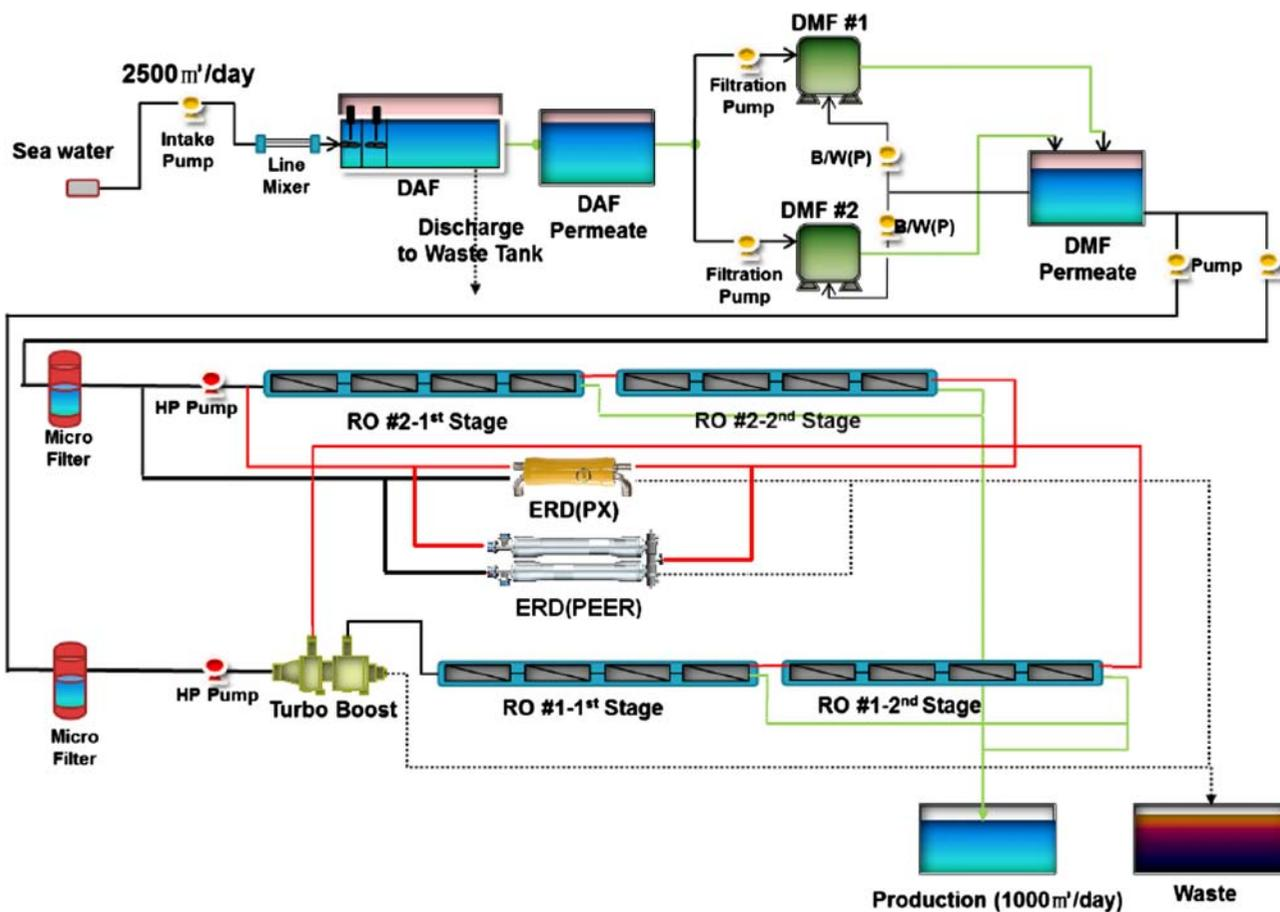
Fig. 1. A schematic diagram of the pilot plant for seawater desalination.
