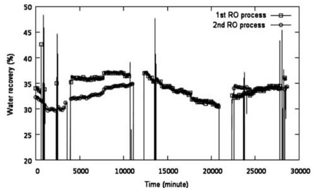
Fig. 3. Identification of operation status on the RO processes by water recovery.
