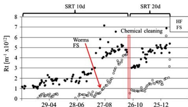
Fig. 2. Total resistance evolution of the flat sheet module (FS) and the hollow fibre module (HF) of the IFAS-MBR.
