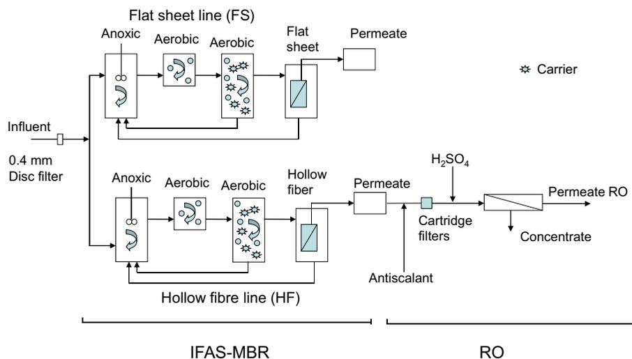
Fig. 1. Scheme of the advanced treatment process for wastewater reclamation.
