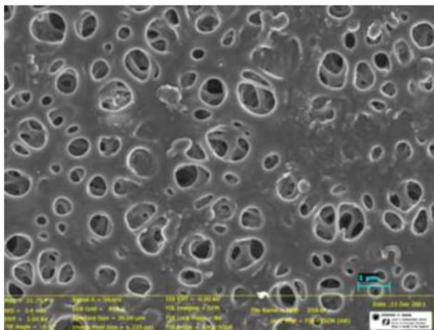
Fig. 4. Flat sheet membrane, clean area.
