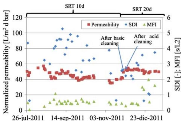
Fig. 8. Permeability evolution of the RO system.
