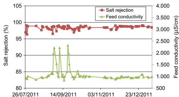
Fig. 9. Feed conductivity and salt rejection of the RO system.
