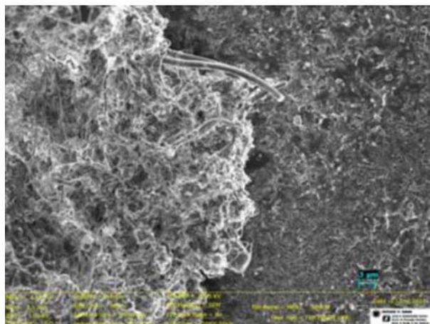
Fig. 5. Flat sheet membrane, fouled area.
