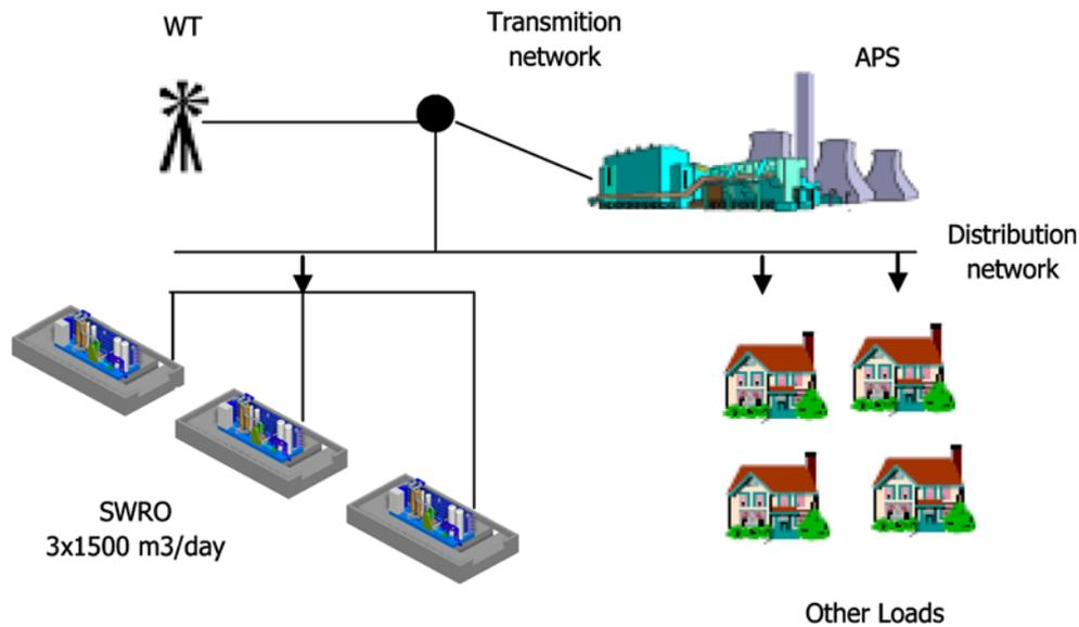
Fig. 5. Schematic diagram of the examined system.
