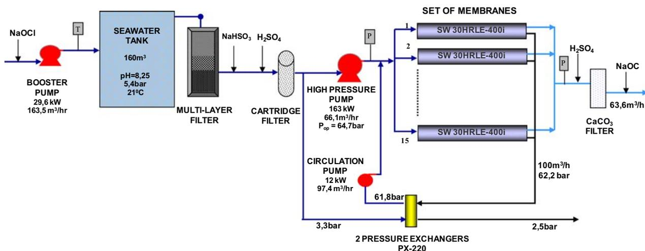
Fig. 4. Flow diagram of the SWRO unit, Mykonos island.
