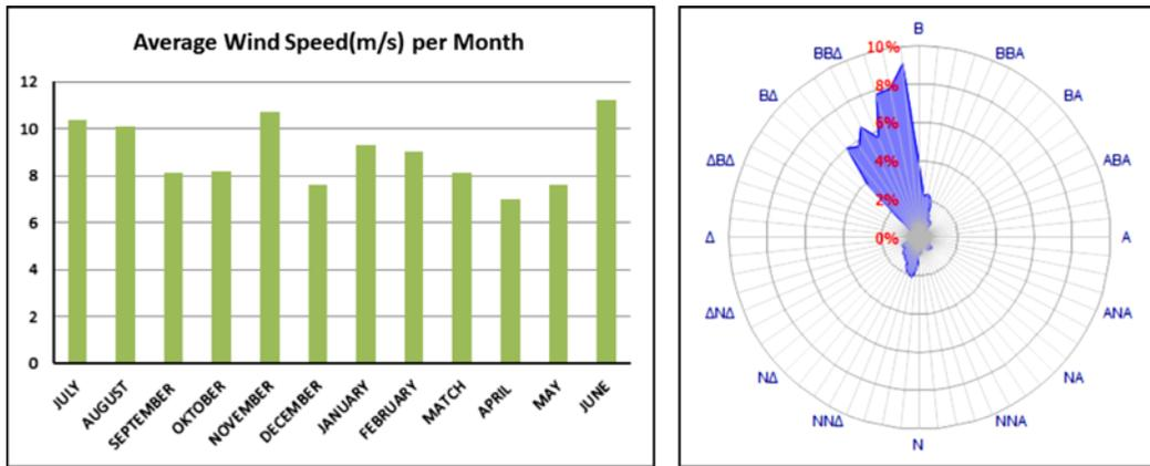
Fig. 7. Measured wind speeds per month and annual wind direction.
