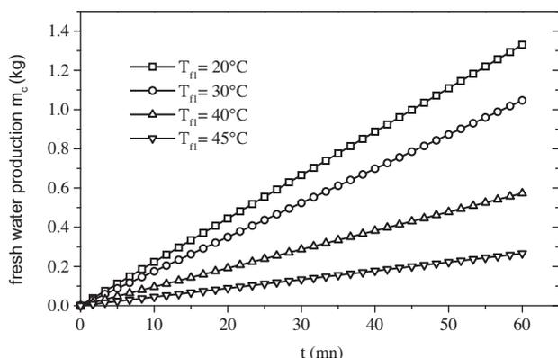
Fig. 6. Effect of inlet cooling water temperature on fresh water production  $m_f = 0.1 \text{ kg/s}$ ,  $m_g = 0.2 \text{ kg/s}$ ,  $T_{g2} = 50^\circ\text{C}$ , and  $W_{g2} = 87.537 \text{ g/kg}$ .
