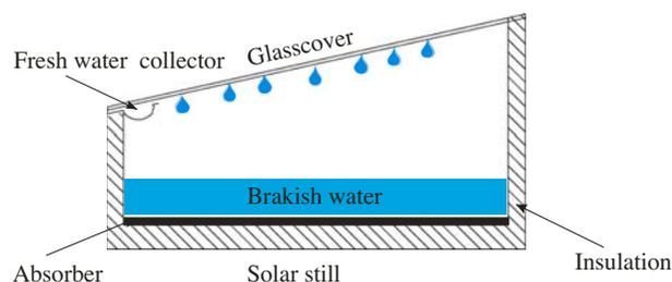
Fig. 1. Schematic representation of the conventional solar still.
