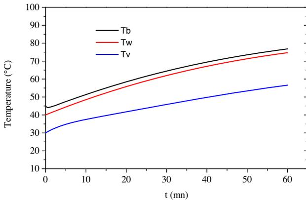
Fig. 3. Temperature variation of different elements of the solar still only.
