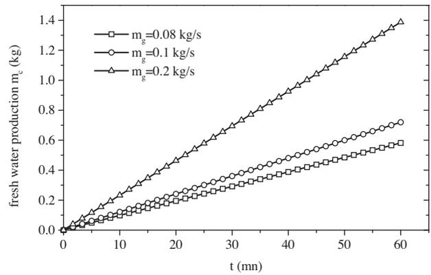
Fig. 5. Effect of moist air flow rate on fresh water production  $m_f = 0.1 \text{ kg/s}$ ,  $T_{f1} = 20 \text{ }^\circ\text{C}$ ,  $T_{g2} = 50 \text{ }^\circ\text{C}$ , and  $W_{g2} = 87.537 \text{ g/kg}$ .
