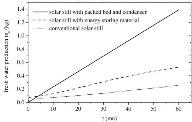
Fig. 4. Comparison of fresh water production.
