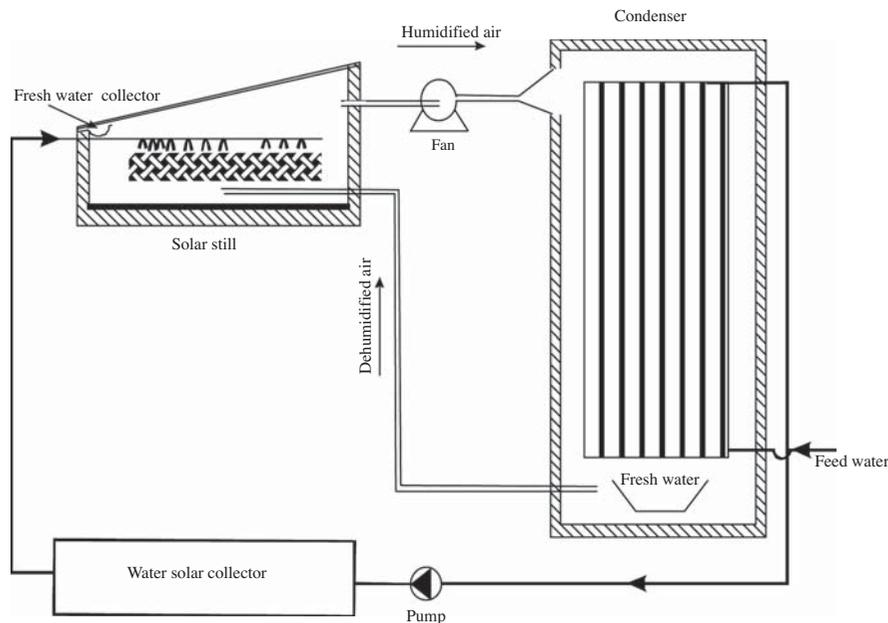
Fig. 2. The proposed desalination system.
