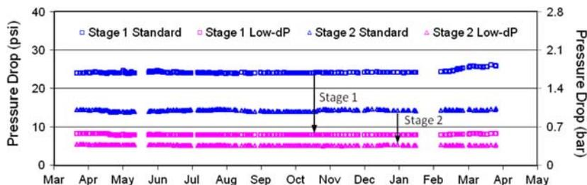
Fig. 7. Side-by-side trial of two feed spacers in a municipal water application—comparison of feed side pressure drop.
