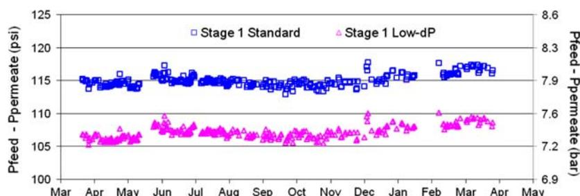
Fig. 8. Side-by-side trial of two feed spacers in a municipal water application—comparison of net applied pressure.
