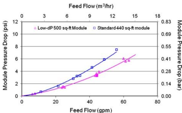
Fig. 9. Comparison of feed-side pressure drop for 8-inch diameter modules with 440 and 500 ft<sup>2</sup> of membrane active area.
