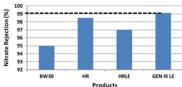
Fig. 2. Nitrate rejection (150 ppm) for different DOW membranes.
