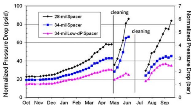
Fig. 6. Side-by-side comparison of three feed spacers in an industrial water application using a conventionally-pretreated, high-fouling feed.
