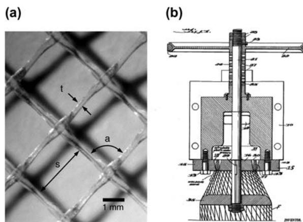
Fig. 3. (a) Biplanar extruded netting is comprised of two intersecting sets of parallel, extruded strands. (b) An early patent was obtained by Nalle [2].
