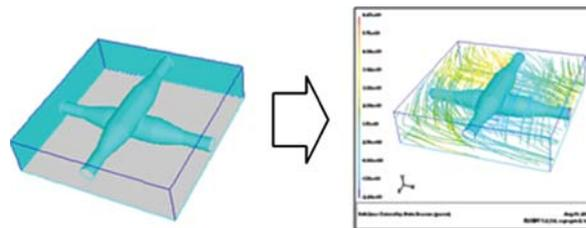
Fig. 5. Three-dimensional models of the feed spacer were used to optimize the tradeoff between pressure drop and mixing.
