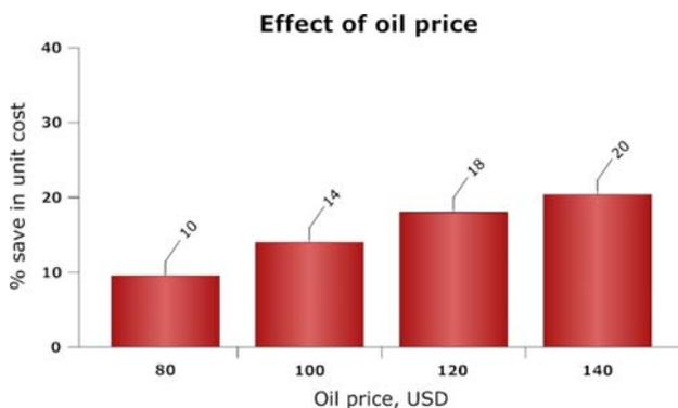
Fig. 8. Effect of oil price on the water unit cost.
