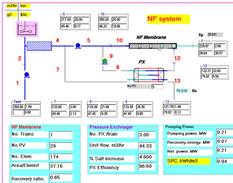
Fig. 3. VDS interface of NF system with pressure exchanger.
