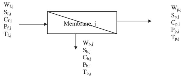
Fig. 2. Schematic diagram of the NF membrane streams.
