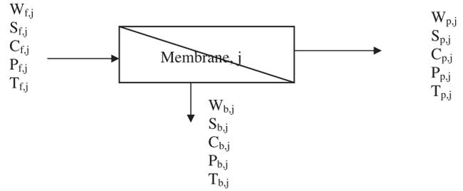
Fig. A1. Schematic diagram of the NF membrane streams.
