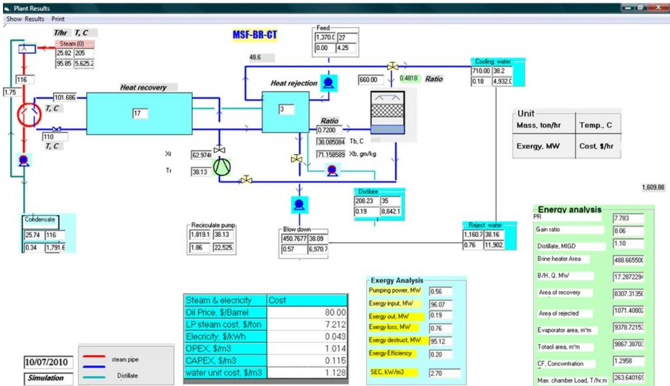
Fig. 4. Interface of existing MSF-BR desalination plant at TBT = 110°C.
