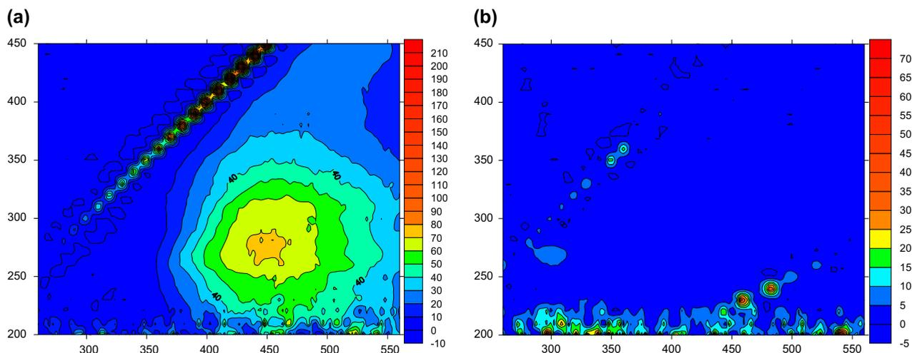
Fig. 6. Scanning of fluorescence of 6 mg/L HA feed solution; (a) At the beginning of the experiment in feed solution, (b) After text in draw solution.
