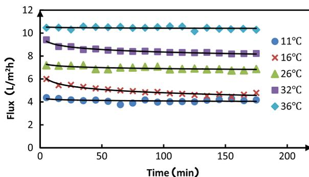
Fig. 3. Effect of temperature on FO permeate flux.
