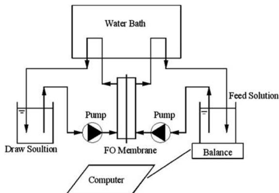
Fig. 1. Schematic diagram of a laboratory-scale FO set-up.
