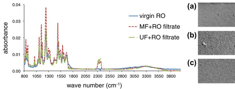
Fig. 7. FTIR spectra and SEM images comparing virgin/filtrated RO membranes. SEM photos: (a) virgin RO membrane (top), (b) RO membrane after filtration of MF filtrate (middle), and (c) RO membrane after filtration of UF filtrate (bottom).
