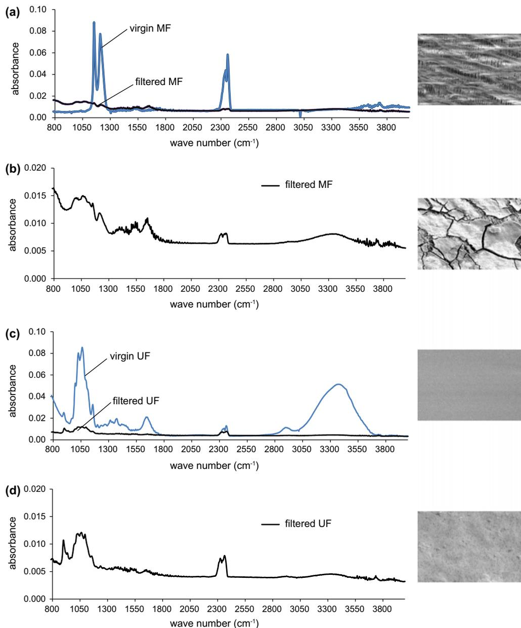
Fig. 4. FTIR spectra and SEM images (a) virgin and filtered MF membranes, (b) enlarged figure of filtered MF membrane, (c) virgin and filtered UF membranes, and (d) enlarged figure of filtered UF membrane.
