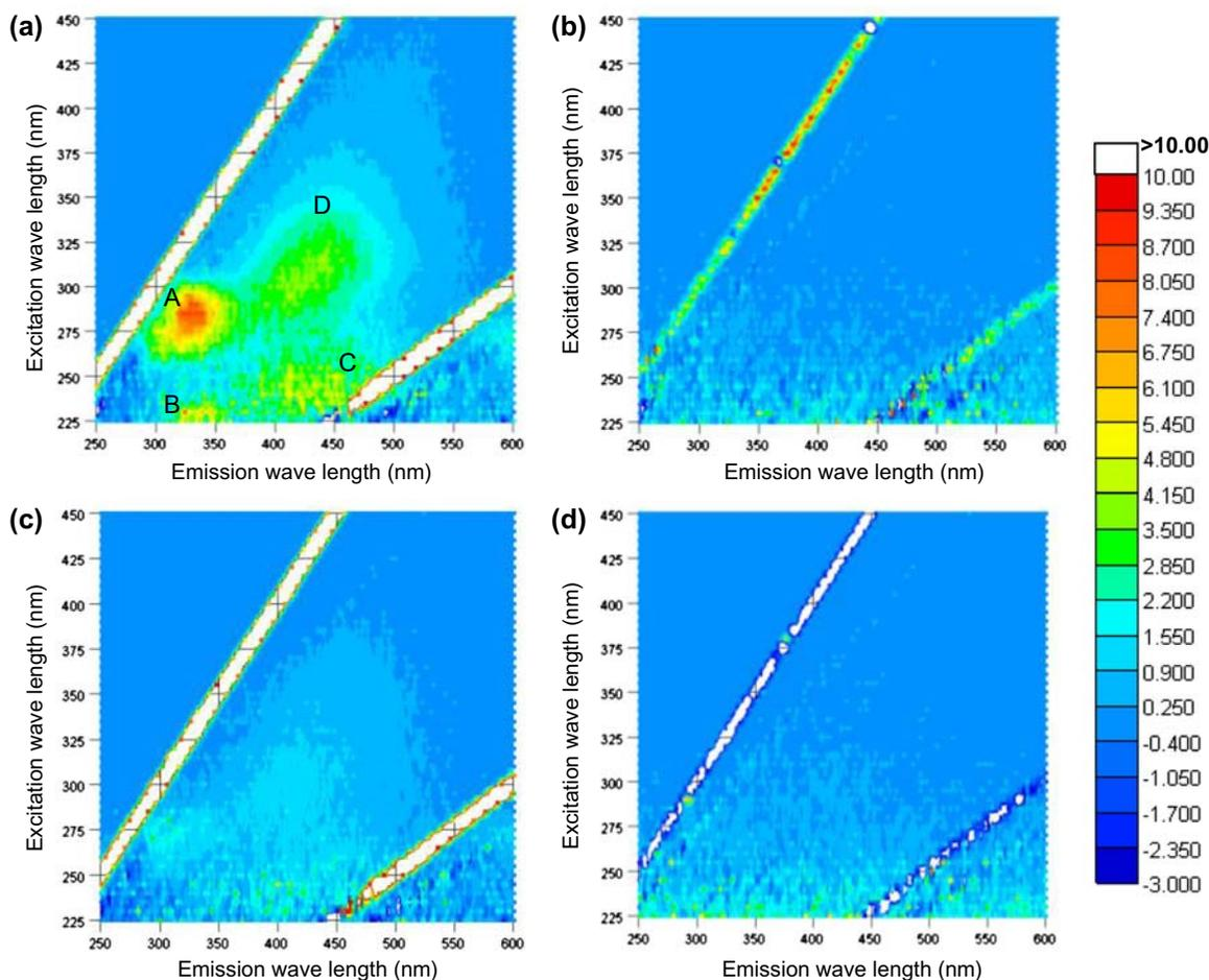
Fig. 6. EEM fluorescence spectra of each step (a) Brine of MF filtrate, (b) RO filtrate of (a), (c) Brine of UF filtrate, and (d) RO filtrate of (c).
