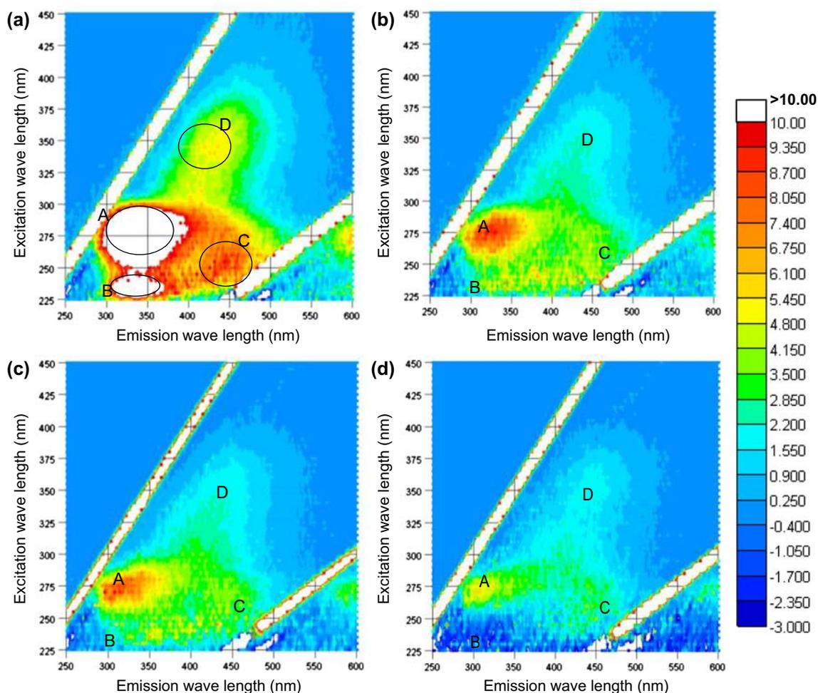
Fig. 2. EEM fluorescence spectra of (a) *C. polykrikoides* culture, (b) Supernatant (after coagulation), (c) MF filtrate, and (d) UF filtrate.
