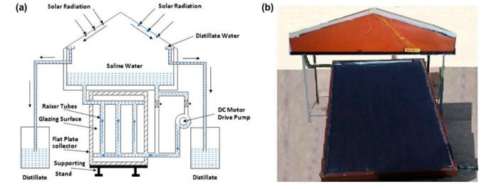
Fig. 1. (a) Cross-sectional view of a double slope active solar still and (b) double slope active solar still set up.
