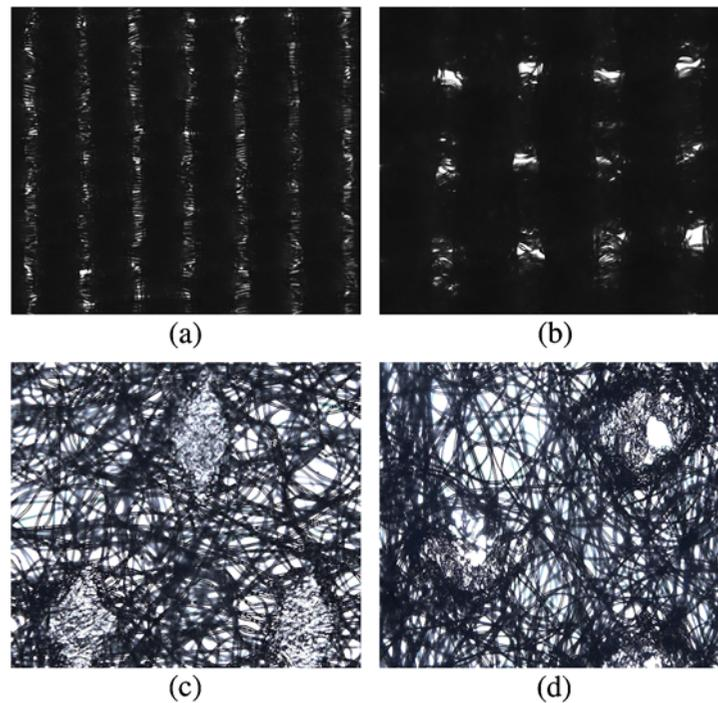
Fig. 1. Microscopic images of surface voids of (a) PA, (b) PES, (c) PP and (d) bicomponent PP/PE; enlarged five times.
