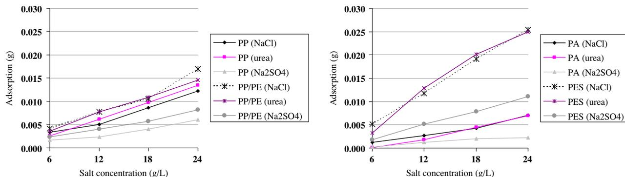
Fig. 2. The amount of adsorbed salt on nonwoven textiles (left) and woven textiles (right).
