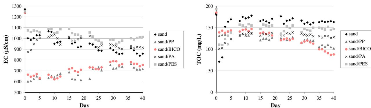
Fig. 3. Electrical conductivity (left) and TOC (right) in initial and treated wastewater.
