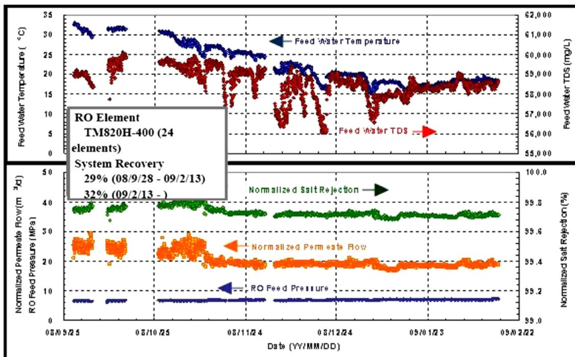
Fig. 4. Performance data of an RO system.
