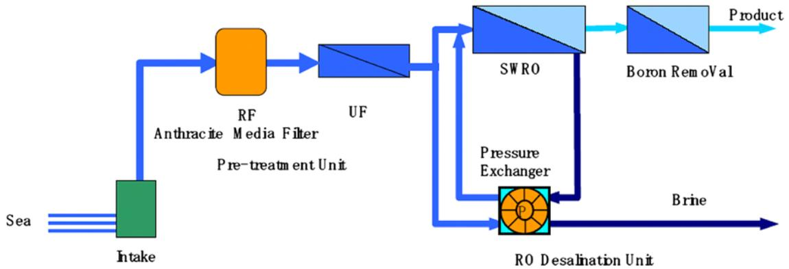
Fig. 2. A schematic process diagram of the demonstration plant at Dukhan.
