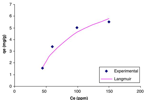
Fig. 6. Adsorption isotherm of chloride ion onto Amberlite IRA-402 fitted by Langmuir isotherm at pH = 9 and T = 25°C.
