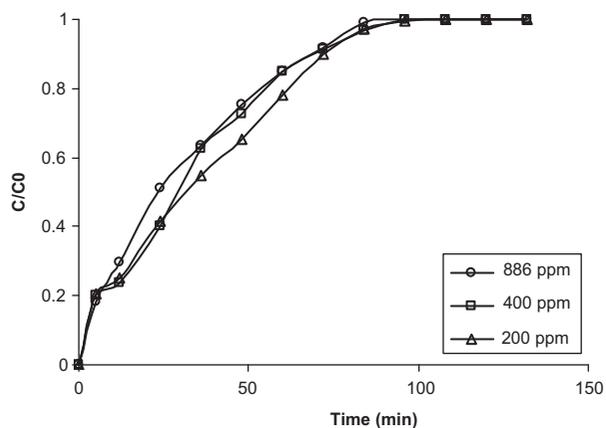
Fig. 14. Effect of influent chloride concentration on the breakthrough curves at bed height = 12 cm,  $Q=50$  ml/min,  $\text{pH}=7.3$  and  $T=25^\circ\text{C}$ .
