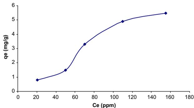
Fig. 2. Adsorption isotherm of chloride ions from the solution onto Amberlite IRA-402 at pH=7.3 and  $T=25^{\circ}\text{C}$ .
