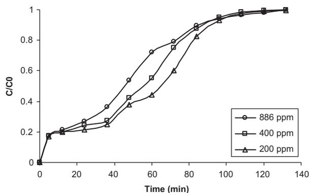
Fig. 13. Effect of influent chloride concentration on the breakthrough curves at bed height = 22 cm,  $Q=50$  ml/min,  $\text{pH}=7.3$  and  $T=25^\circ\text{C}$ .
