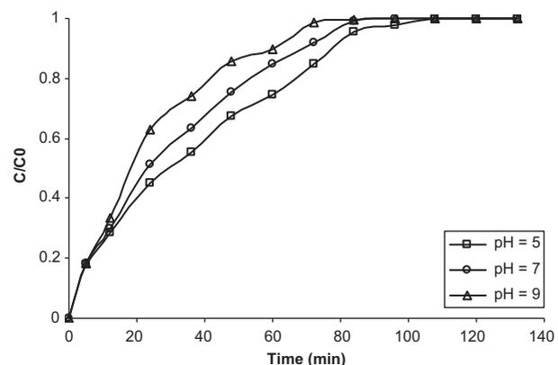
Fig. 9. Effect of feed initial pH on the breakthrough curves at bed height 12 cm,  $C_0 = 886$  ppm,  $Q = 50$  ml/min and  $T = 25^\circ\text{C}$ .
