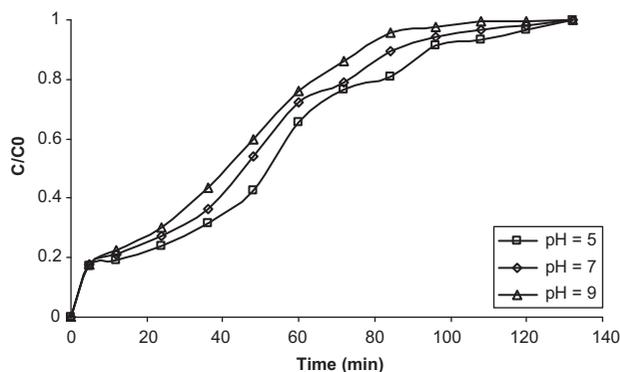
Fig. 8. Effect of feed initial pH on the breakthrough curves at bed height of 22 cm,  $C_0 = 886$  ppm,  $Q = 50$  ml/min and  $T = 25^\circ\text{C}$ .
