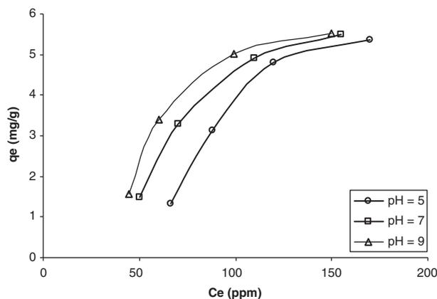
Fig. 5. Effect of initial pH on chloride uptake.
