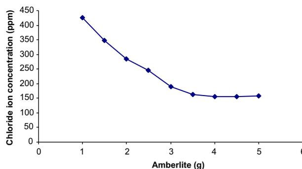
Fig. 1. The chloride ion concentration at equilibrium for different amounts of Amberlite IRA-402 as an adsorbent.
