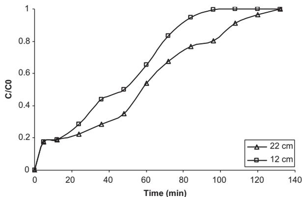
Fig. 15. Adsorption of chloride ion through packed column at  $Q=25$  ml/min  $\text{pH}=7.3$ ,  $C_0=886$  ppm at  $T=25^\circ\text{C}$ .
