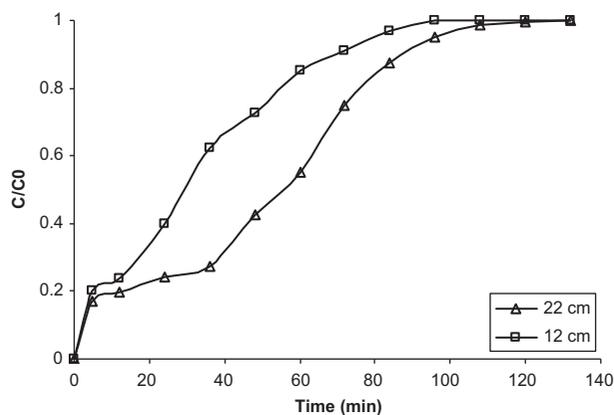
Fig. 11. Adsorption of chloride ion through packed column at  $Q=50$  ml/min,  $\text{pH}=7.3$ ,  $C_0=400$  ppm and  $T=25^\circ\text{C}$ .
