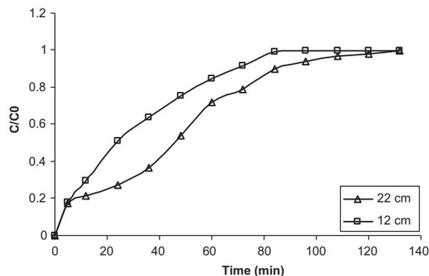
Fig. 10. Adsorption of chloride ion through packed column at  $Q=50$  ml/min,  $\text{pH}=7.3$ ,  $C_0=886$  ppm and  $T=25^\circ\text{C}$ .
