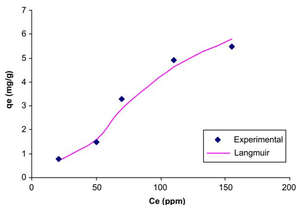
Fig. 3. Langmuir isotherm for chloride adsorption on Amberlite IRA-402 at pH=7.3 and  $T=25^{\circ}\text{C}$ .
