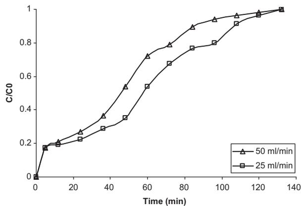
Fig. 16. Effect of influent flow rate on the breakthrough curves at bed height = 22 cm,  $C_0=886$  ppm,  $\text{pH}=7.3$  at  $T=25^\circ\text{C}$ .
