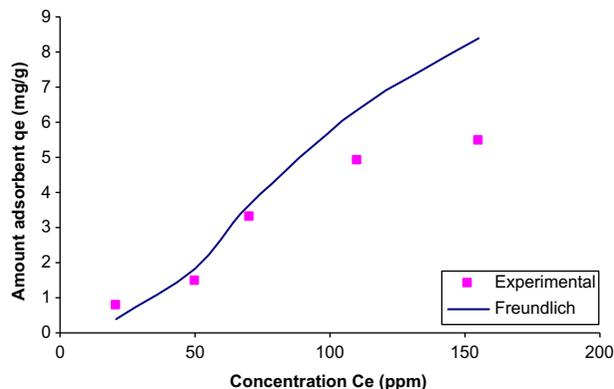
Fig. 4. Freundlich isotherm for chloride adsorption on Amberlite IRA-402 at pH=7.3 and  $T=25^{\circ}\text{C}$ .
