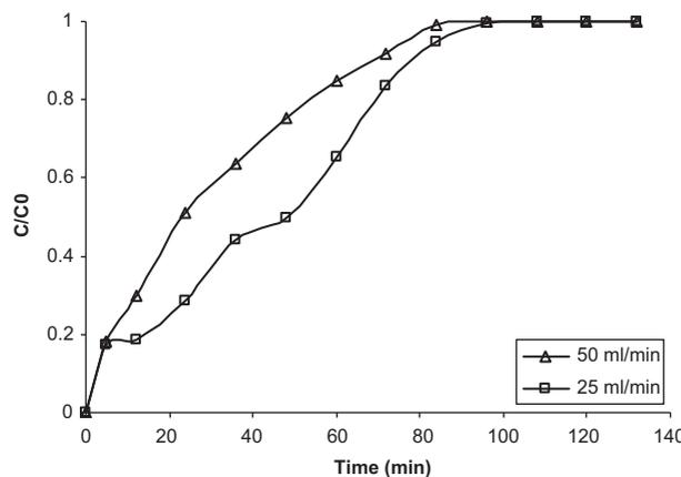
Fig. 17. Effect of influent flow rate on the breakthrough curves at bed height = 12 cm,  $C_0=886$  ppm,  $\text{pH}=7.3$  at  $T=25^\circ\text{C}$ .
