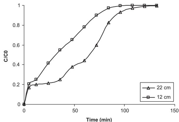
Fig. 12. Adsorption of chloride ion through packed column at  $Q=50$  ml/min,  $\text{pH}=7.3$ ,  $C_0=200$  ppm and  $T=25^\circ\text{C}$ .
