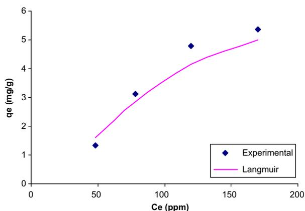
Fig. 7. Adsorption isotherm of chloride ion onto Amberlite IRA-402 fitted by Langmuir isotherm at pH = 5 and T = 25°C.
