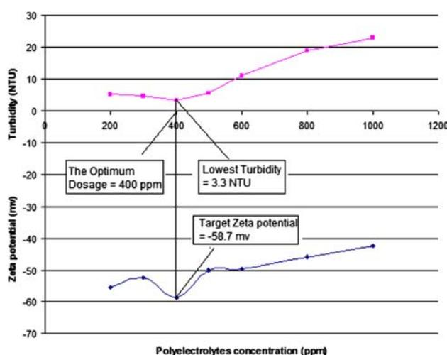
Fig. 3. Polyelectrolyte optimum dosage having the lowest turbidity and target zeta potential.
