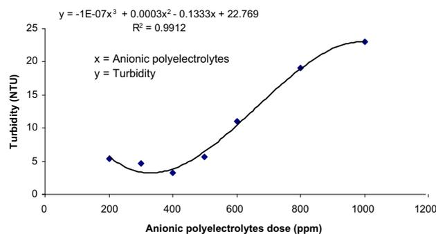
Fig. 2. The turbidity of the clear solution as a function of polyelectrolyte dosage.
