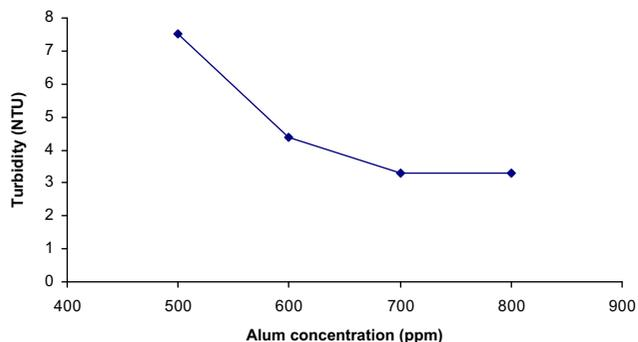
Fig. 5. Turbidity vs. alum dosage after 2 h of initial sedimentation: optimum dosage: 700 ppm.
