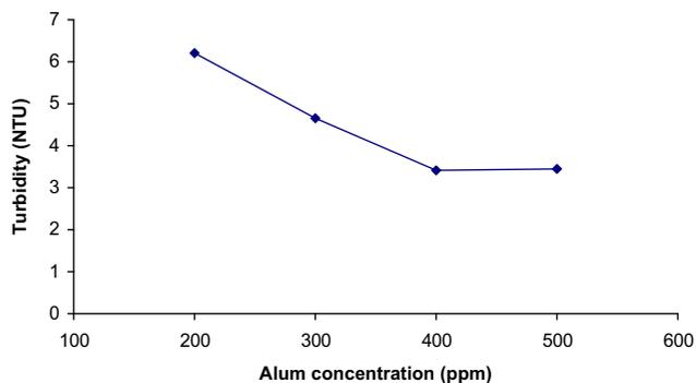
Fig. 6. Turbidity vs. alum dosage after 3 h of initial sedimentation: Optimum dosage: 400 ppm.
