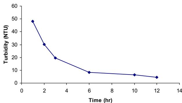
Fig. 1. The turbidity variation with time of wastewater due to sedimentation.
