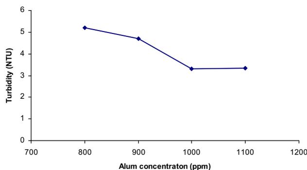
Fig. 4. Turbidity vs. alum dosage after 1 h of initial sedimentation: optimum dosage: 1,000 ppm.
