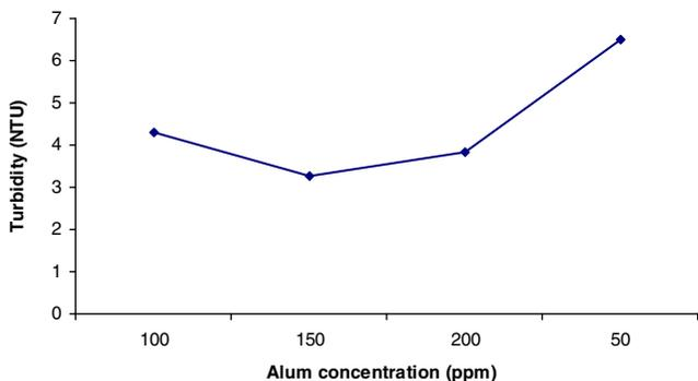
Fig. 7. Turbidity vs. alum dosage after 6 h of initial sedimentation: optimum dosage: 150 ppm.
