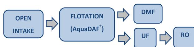
Fig. 1. Flow diagram of the pilot treatment line.
