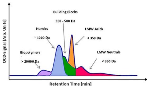
Fig. 2. LC-OCD fractions over the SEC chromatogram with OCD.
