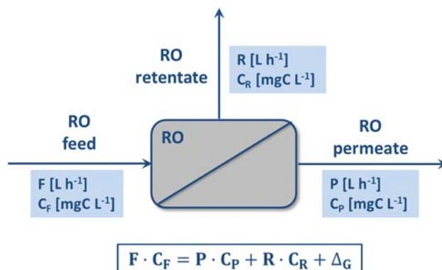
Fig. 4. RO unit operation and mass balance.
