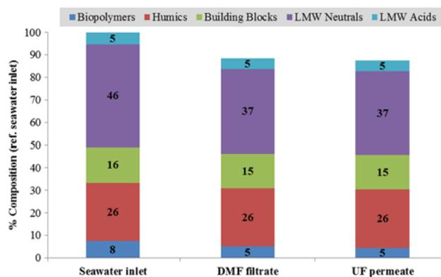
Fig. 3. Seawater inlet, DMF filtrate, and UF permeate composition.
