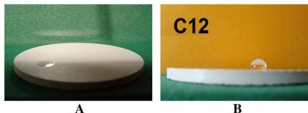
Fig. 7. Behavior of water drop on a surface of  $\text{TiO}_2$  ceramic membranes: (A) unmodified membrane and (B) membrane modified by C12 compounds.
