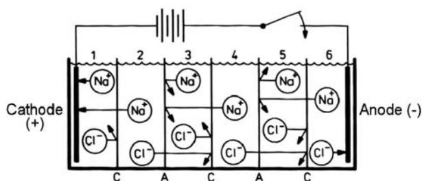
Fig. 4. Electrodialysis [22].
