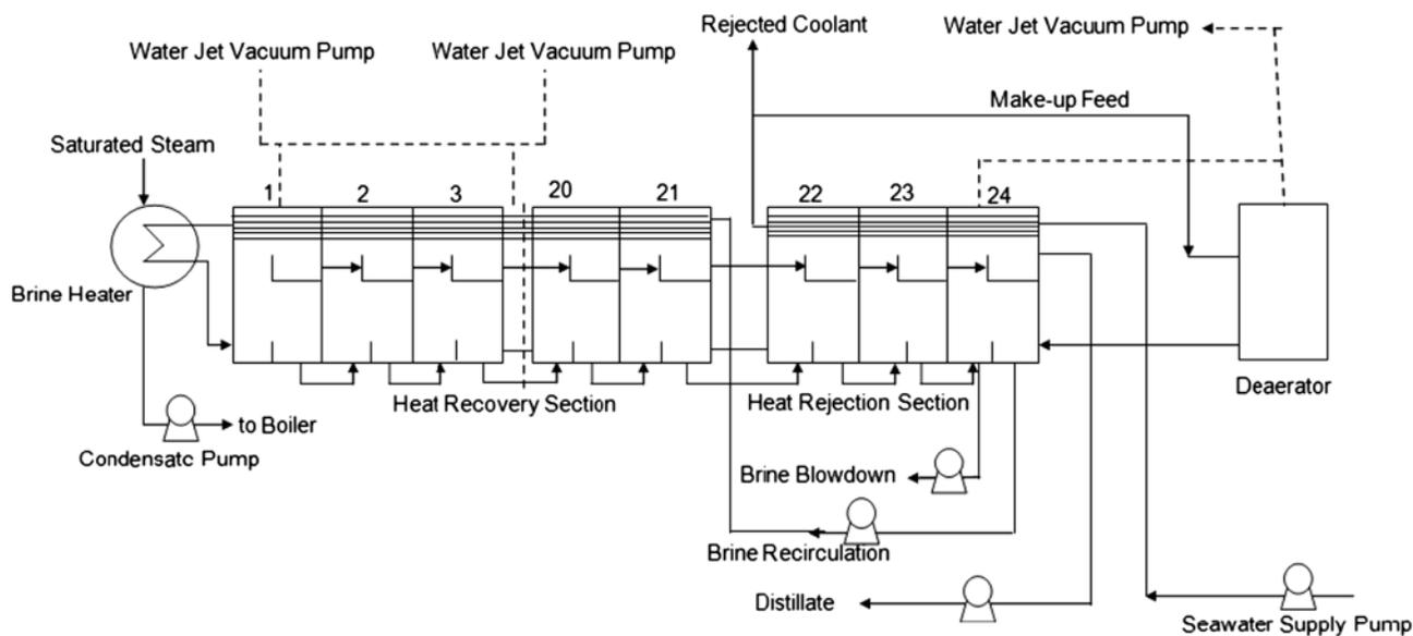
Fig. 1. MSF desalination unit [11].
