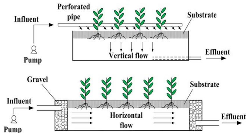
Fig. 1. Schematic diagram of the studied VFCW and HFCW system.
