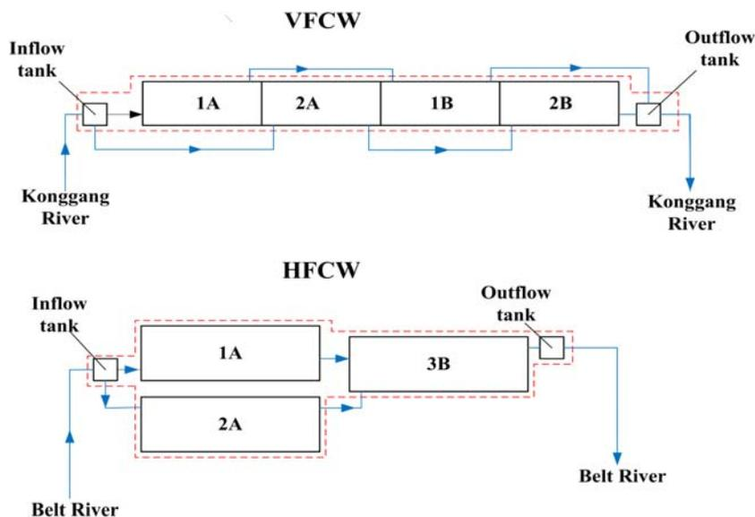
Fig. 2. Pan view and process chart of the studied VFCW and HFCW system.
