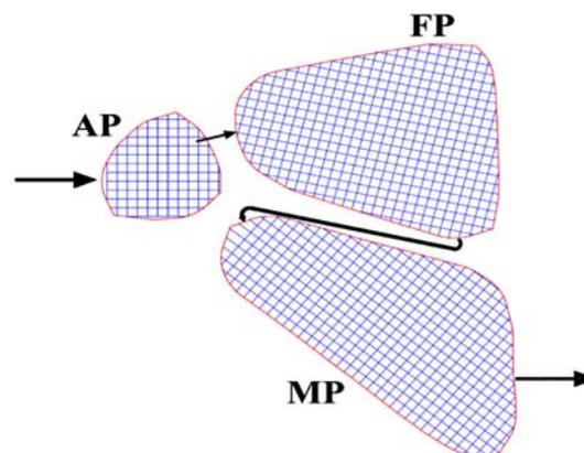
Fig. 1. Schematic representation of ponds and pre-prepared grid established for sludge distribution study. AP= Anaerobic Pond; FP=Facultative Pond; MP=Maturation Pond.
