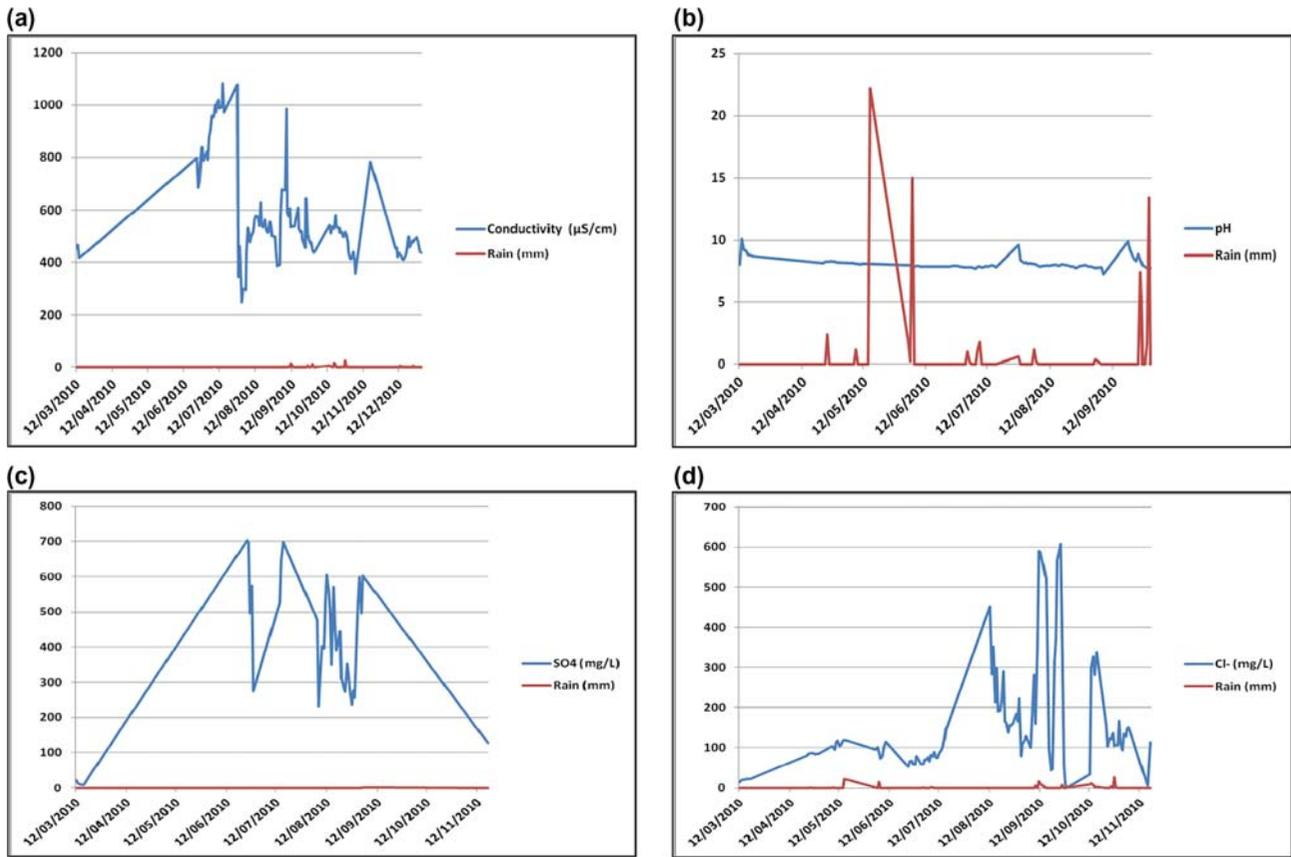
Fig. 9. (a) Conductivity; (b) pH; (c)  $\text{SO}_4^{2-}$ ; and (d)  $\text{Cl}^-$  daily average values vs rainfall from “Soulou” stream monitoring station (0033).
