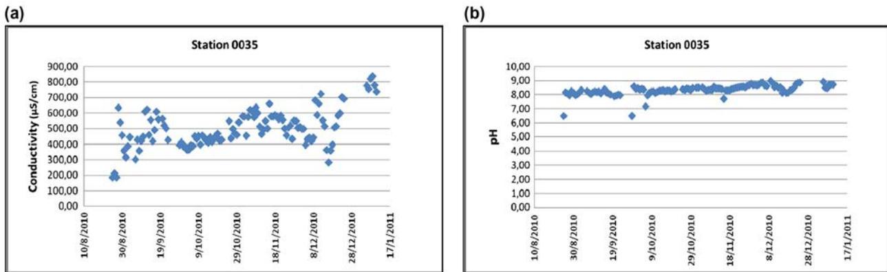
Fig. 8. (a) Conductivity and (b) pH daily average measured values vs time from “Ag. Dimitrios” PPC monitoring station (0035).
