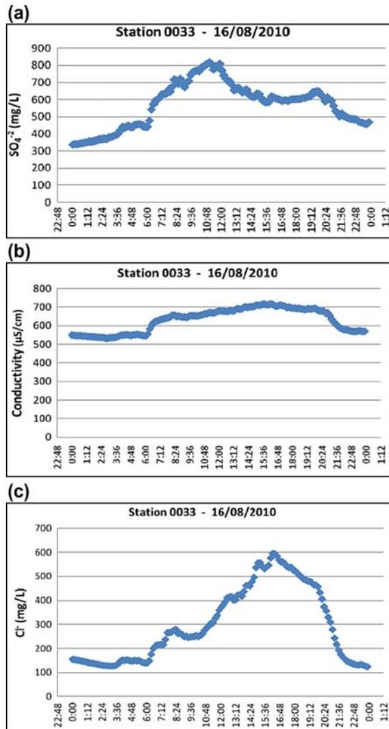
Fig. 5. (a)  $\text{SO}_4^{2-}$ ; (b) conductivity; and (c)  $\text{Cl}^-$  measurements on 16 August 2010 from “Soulou” stream monitoring station (0033).
