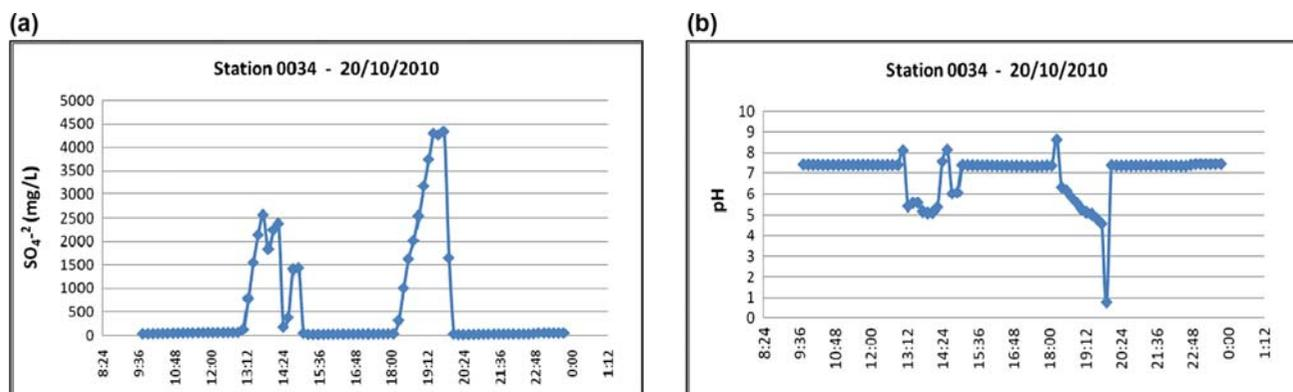
Fig. 7. (a)  $\text{SO}_4^{2-}$  and (b) pH measured values on 20 October 2010 from “drilling” monitoring station (0034).
