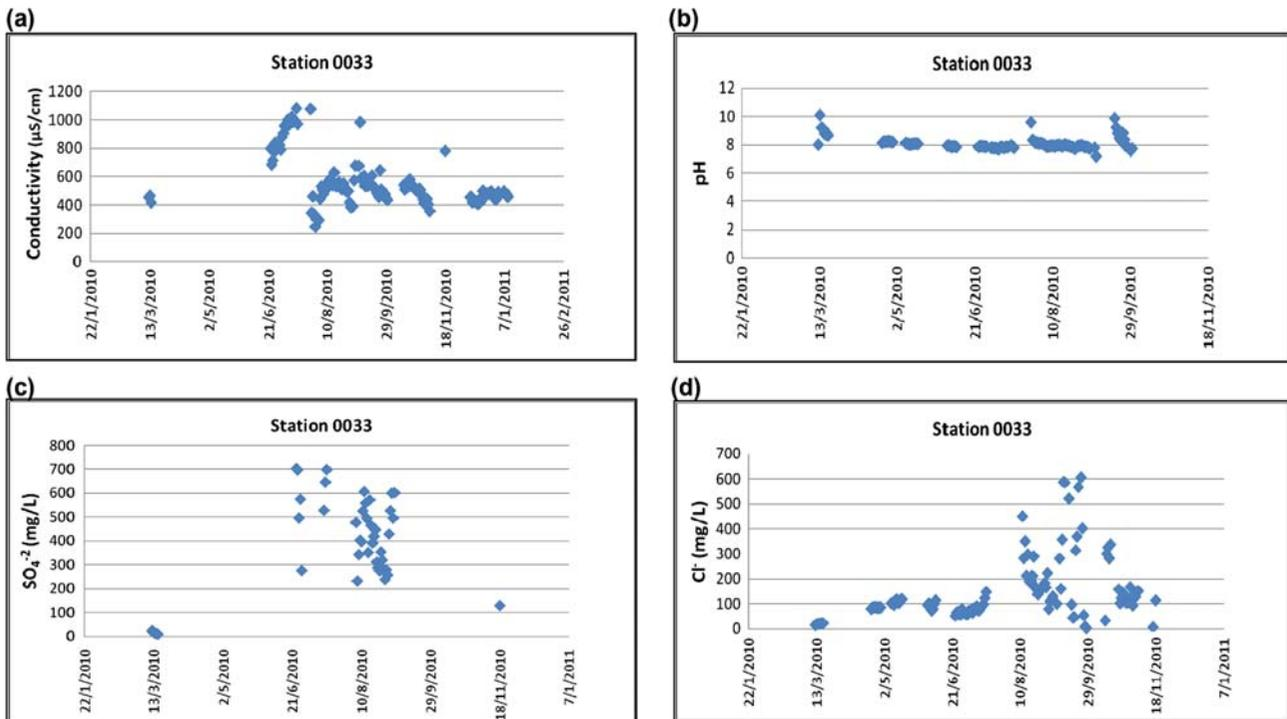
Fig. 4. (a) Conductivity; (b) pH; (c)  $\text{SO}_4^{2-}$ ; and (d)  $\text{Cl}^-$  daily average values vs time from “Soulou” stream monitoring station (0033).
