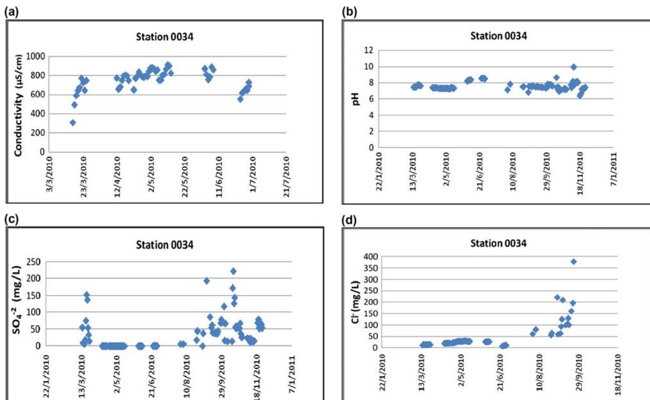
Fig. 6. (a) Conductivity; (b) pH; (c)  $\text{SO}_4^{2-}$ ; and (d)  $\text{Cl}^-$  daily average measured values vs time from “drilling” monitoring station (0034).
