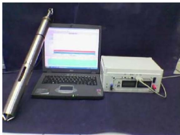
Fig. 1. The multi-parameter sensors system (Watertool II).
