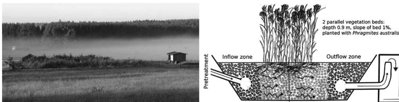
Fig. 1. Diagram and photograph of the subsurface horizontal flow CW in Slavošovice, Czech Republic.
