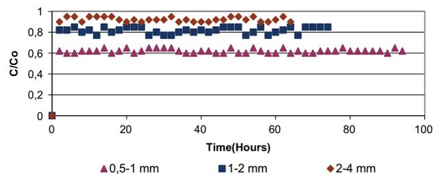
Fig. 4. The comparison of suspended solids removal performances.
