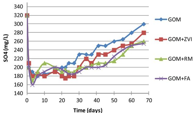
Fig. 5. Evolution of  $\text{SO}_4$  concentration in effluents vs. time.
