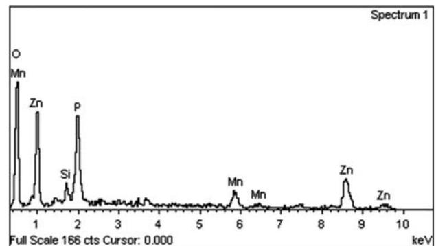
Fig. 6b. Element spectrum of “exhausted” GOM seen in Fig. 6a.
