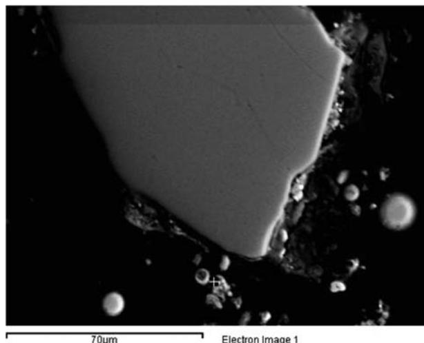
Fig. 8a. SEM-BSI of “exhausted” GOM + FA mixture, scale 70  $\mu\text{m}$ .
