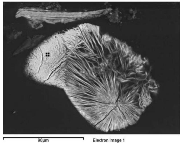
Fig. 6a. SEM-BSI of “exhausted” GOM, scale 90  $\mu\text{m}$ .
