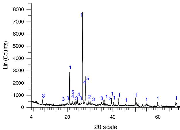
Fig. 4. X-ray pattern of “exhausted” GOM (1: quartz— $\text{SiO}_2$ , 2: calcite— $\text{CaCO}_3$ , 3: illite— $(\text{K},\text{H}_3\text{O})(\text{Al},\text{Mg},\text{Fe})_2(\text{Si},\text{Al})_4\text{O}_{10}[(\text{OH})_2,(\text{H}_2\text{O})]$ , 4: albite— $\text{NaAlSi}_3\text{O}_8$  and 5: covellite— $\text{CuS}$ ).
