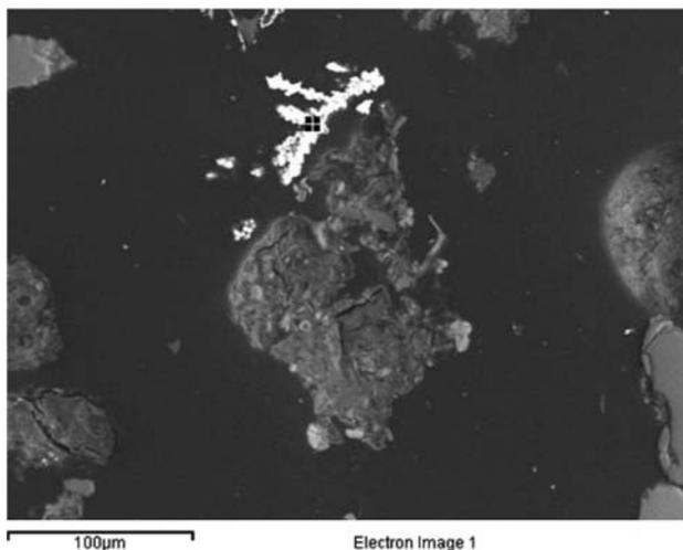
Fig. 7a. SEM-BSI of “exhausted” GOM + ZVI mixture, scale 100  $\mu\text{m}$ .
