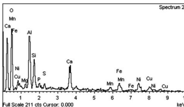
Fig. 8b. Element spectrum of “exhausted” GOM + FA mixture seen in Fig. 8a.
