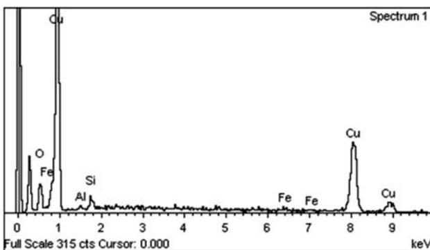
Fig. 7b. Element spectrum of “exhausted” GOM + ZVI mixture seen in Fig. 7a.
