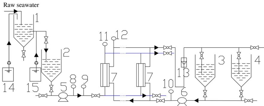
Fig. 5. Flow diagram of ceramic membrane system. (1) blend tank; (2) feed tank; (3) permeate tank; (4) cleaning tank; (5) feed pump; (6) backwashing pump; (7) ceramic membrane modules; (8) temperature transducer; (9,10,11,12) pressure transducers; (13) flow transducer; (14) metering pump for FeCl<sub>3</sub>; (15) metering pump for NaClO.
