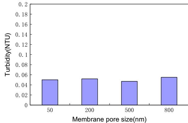
Fig. 10. Effect of ceramic membrane pore size on the turbidity of permeates.
