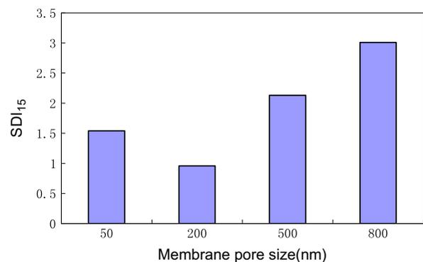
Fig. 11. Effect of membrane pore size on the  $SDI_{15}$  value of permeates.
