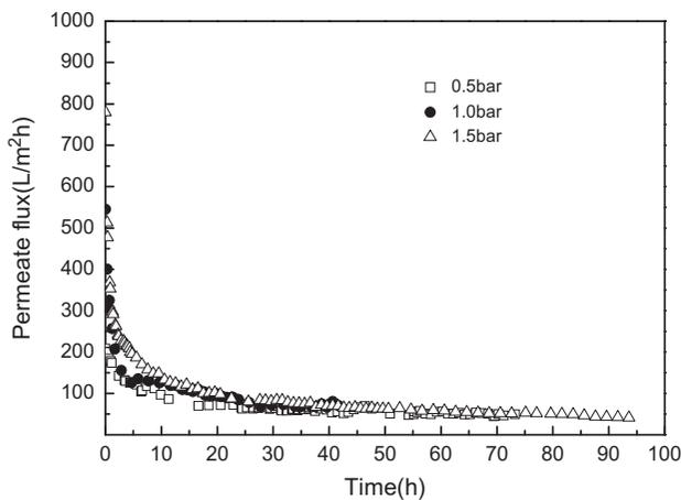
b. Membrane pore size of 200 nm
