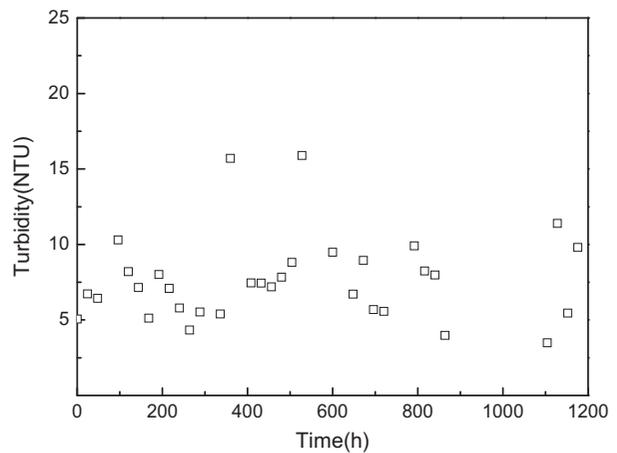
Fig. 14. Turbidity of the feed for the ceramic membrane device.
