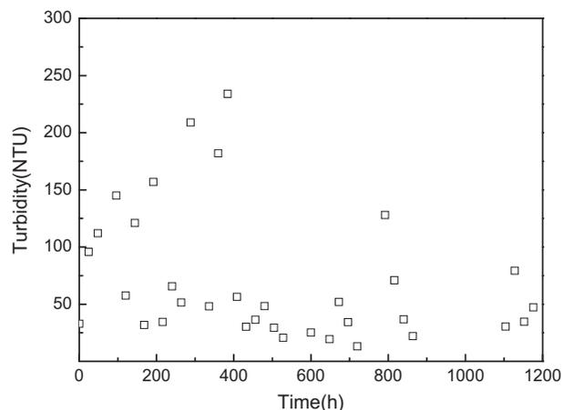
Fig. 2. Turbidity of the raw seawater.
