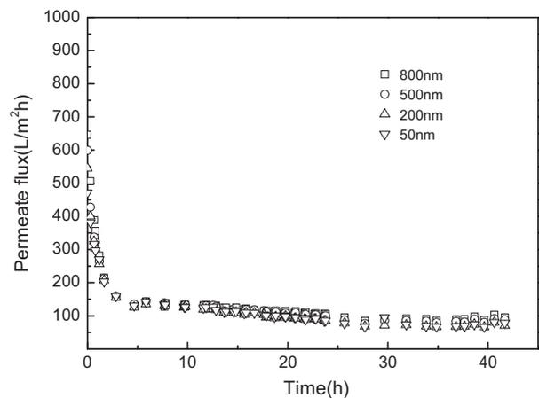
Fig. 6. Permeate fluxes of ceramic membranes with different pore sizes.
