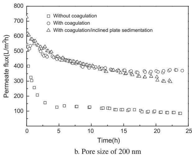
Fig. 9. Performance of the ceramic membrane filtering seawater with different treatments.
