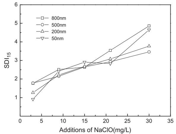
Fig. 13. Effect of NaClO addition on the SDI<sub>15</sub> values of permeates.
