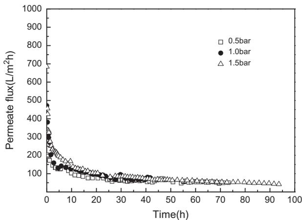
a. Membrane pore size of 50 nm
