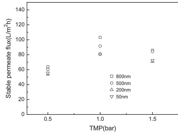
Fig. 8. Effect of TMP on the steady state fluxes of the ceramic membranes.
