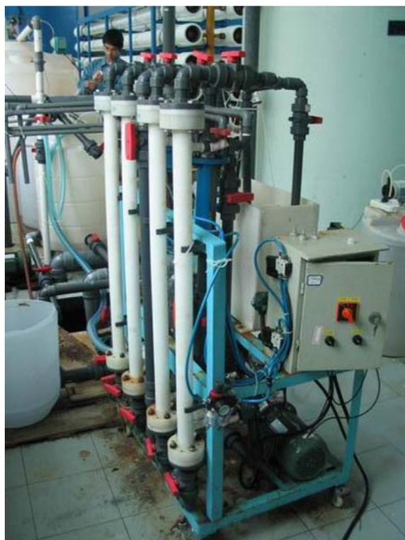
Fig. 3. Experimental setup of the ceramic membrane filtration system.
