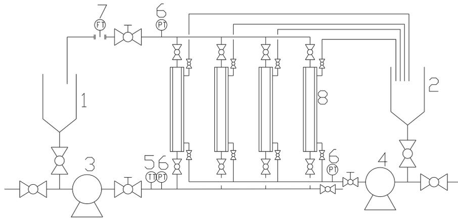
Fig. 4. Flow diagram of laboratory-scale experiment. (1) feed tank; (2) permeate tank; (3) feed pump; (4) backwash pump; (5) thermometer; (6) pressure gauges; (7) flowmeter; (8) membrane modules.
