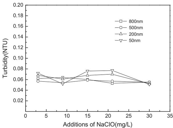
Fig. 12. Effect of NaClO addition on the turbidities of permeates.
