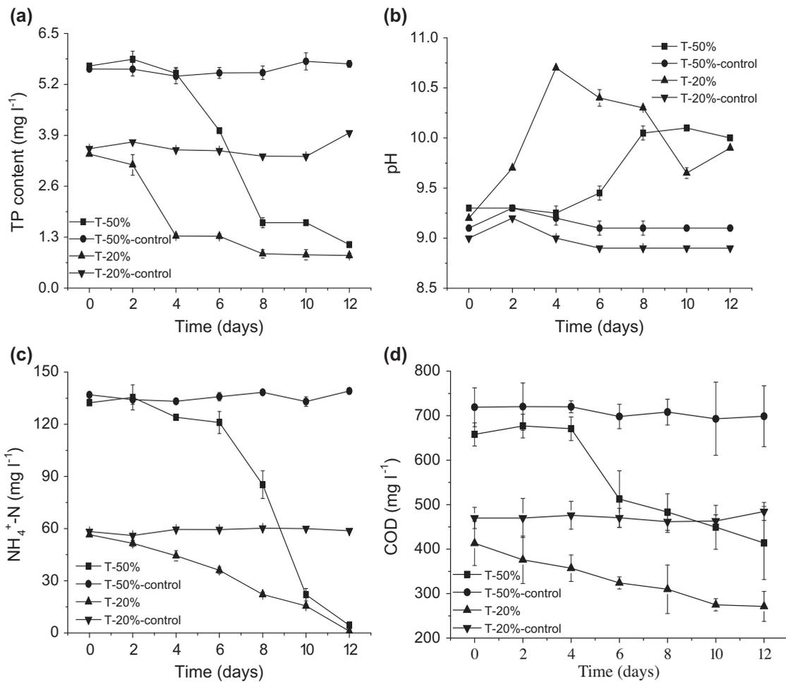
Fig. 4. Changes of TP (a), pH (b),  $\text{NH}_4^+ - \text{N}$  (c), and COD (d) in growth media, respectively (TP: total phosphorus;  $\text{NH}_4^+ - \text{N}$ : ammonia nitrogen; COD: chemical oxygen demand).
