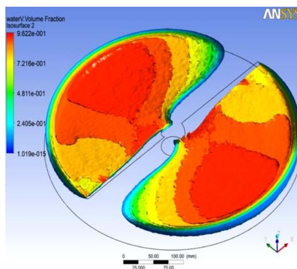
Fig. 5. An example showing the numerical simulation result for supercavitation in a rotating cavitator.
