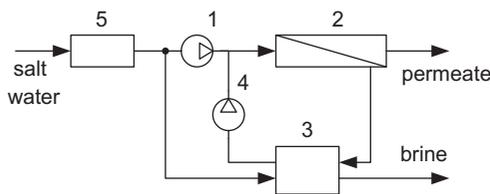
Fig. 4. Reverse osmosis distillation facility: 1—high pressure pump; 2—reverse osmosis membrane; 3—energy recovering device; 4—booster pump; 5—water pre-treatment system.
