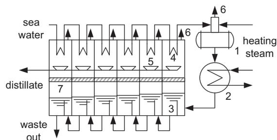
Fig. 2. Multi-stage flash distillation facility: 1—deaerator; 2—brine heater; 3—flashing chamber; 4—condenser coil; 5—condensate collector; 6—to the vacuum system; 7—demister.
