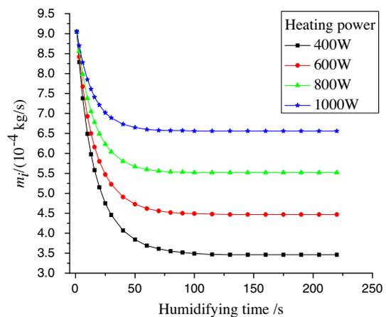
Fig. 5.  $m_i$  changed with time ( $T_1 = 60^\circ\text{C}$ ).
