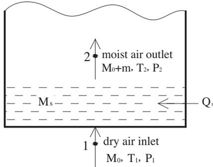
Fig. 3. Schematic diagram of energy balance in humidifier.
