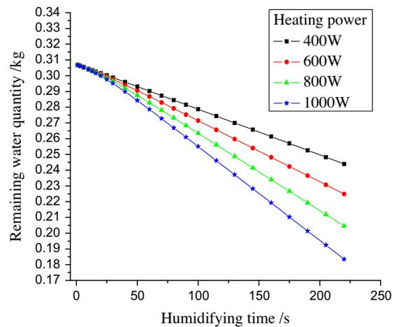
Fig. 12. Water quantity changed with time ( $T_1=40^\circ\text{C}$ ).
