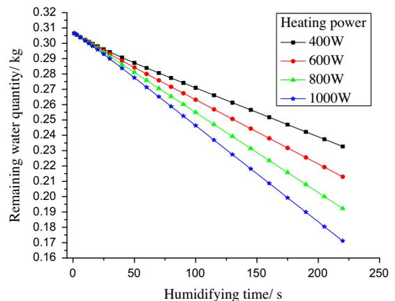
Fig. 10. Water quantity changed with time ( $T_1 = 50^\circ\text{C}$ ).
