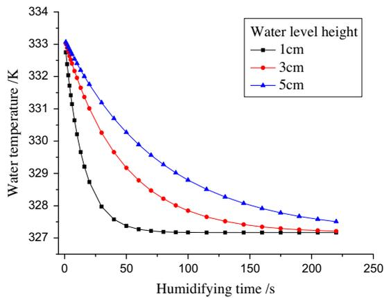
Fig. 13. Water temperature changed with time ( $T_1 = 50^\circ\text{C}$ ).
