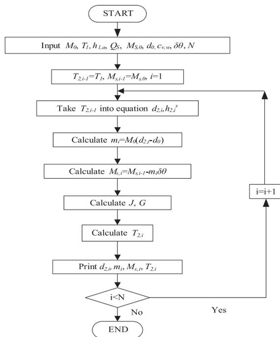
Fig. 4. Calculation flow chart of humidifying process.
