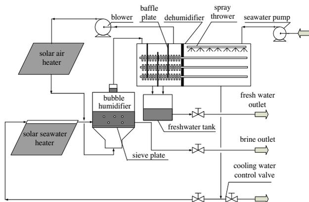
Fig. 1. Solar desalination process by bubbling humidification.
