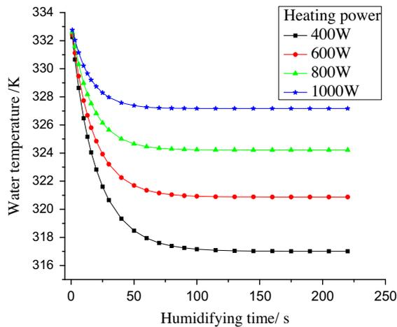
Fig. 6. Water temperature changed with time ( $T_1 = 60^\circ\text{C}$ ).
