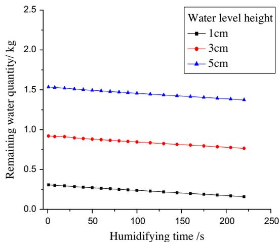
Fig. 14. Water quantity changed with time ( $T_1 = 50^\circ\text{C}$ ).
