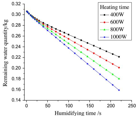
Fig. 7. Water quantity changed with time ( $T_1 = 60^\circ\text{C}$ ).
