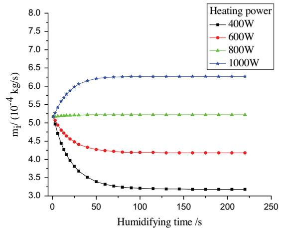
Fig. 8.  $m_i$  changed with time ( $T_1 = 50^\circ\text{C}$ ).
