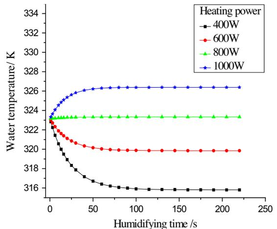
Fig. 9. Water temperature changed with time ( $T_1 = 50^\circ\text{C}$ ).
