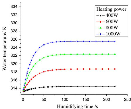
Fig. 11. Water temperature changed with time ( $T_1=40^\circ\text{C}$ ).
