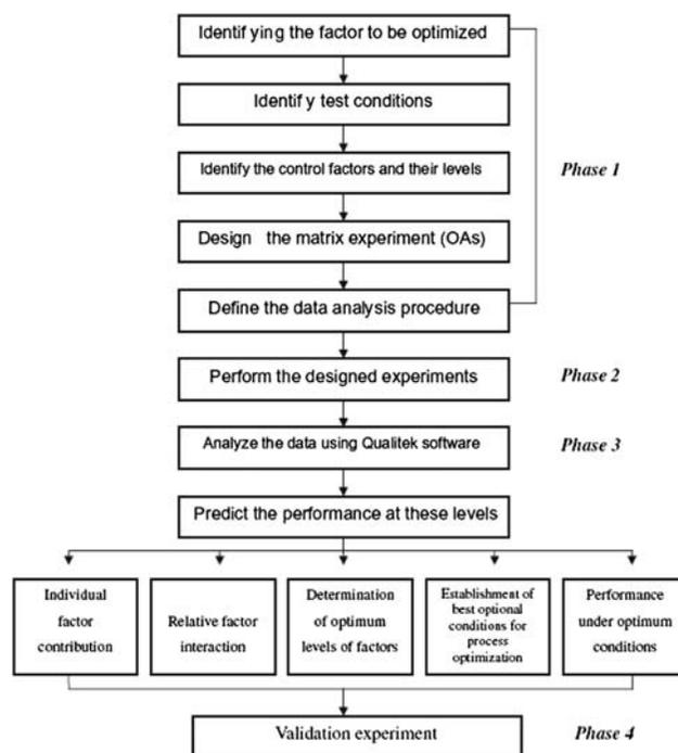
Fig. 1. Schematic representation of the steps involved in the Taguchi DOE methodology.
