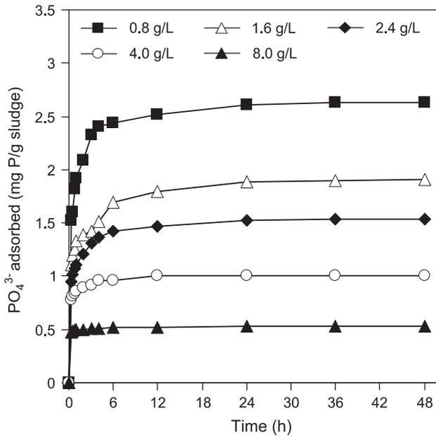
Fig. 2. Kinetic data of phosphate adsorption onto different doses of PAC (0.8–8.0 g/L).
