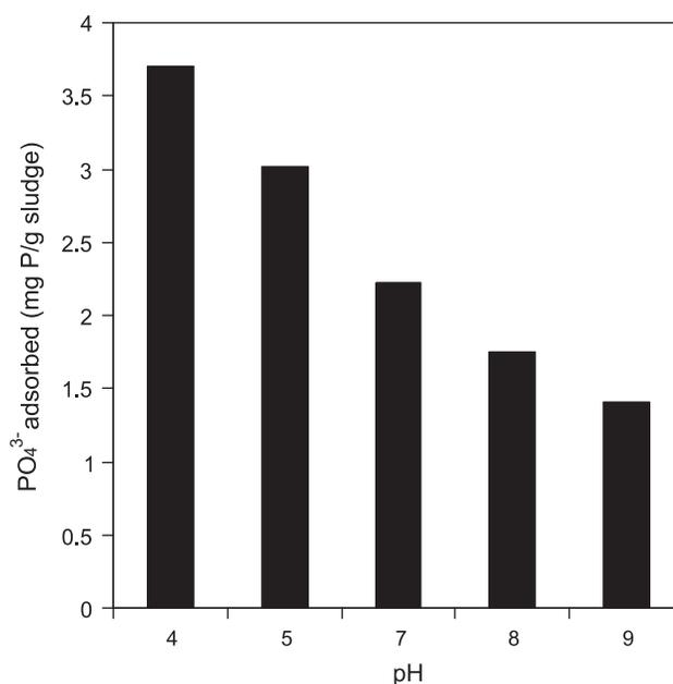
Fig. 5. Effect of pH on phosphate adsorption by PAC sludge.
