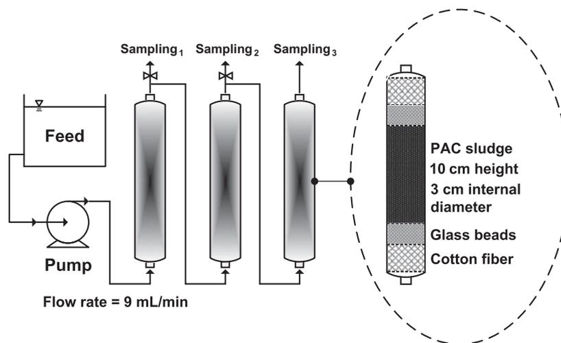
Fig. 1. Schematic diagram of a continuous fixed-bed column experiment.
