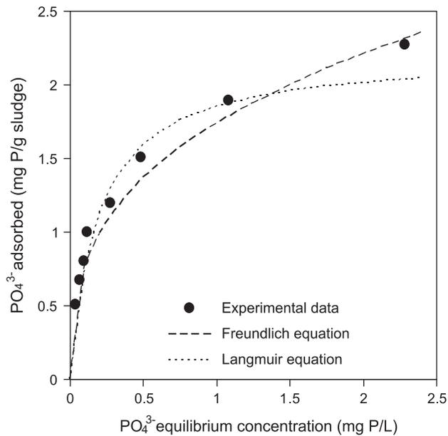
Fig. 3. Phosphate adsorption isotherm for PAC sludge.
