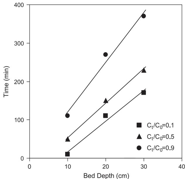
Fig. 7. Service time vs. bed depth for breakthrough at  $C_t/C_0$  ratio 0.1, 0.5, and 0.9.
