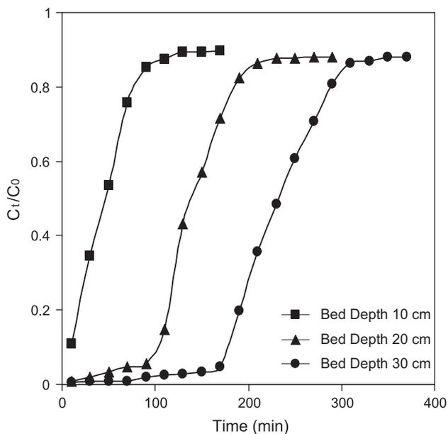
Fig. 6. Breakthrough curves for different bed depths.
