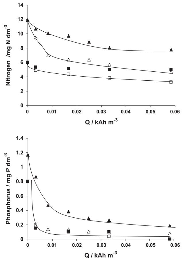
Fig. 5. Influence of the reagent dosed on the removal of nutrients (after 40 μm filtration) by electrocoagulation. WWTP<sub>1</sub> ▲ iron Δ aluminium; WWTP<sub>2</sub> ■ iron □ aluminium. Operation conditions:  $T$ : 25°C; flowrate: 50 dm<sup>3</sup> h<sup>-1</sup>; current density: 10 A m<sup>-2</sup>.
