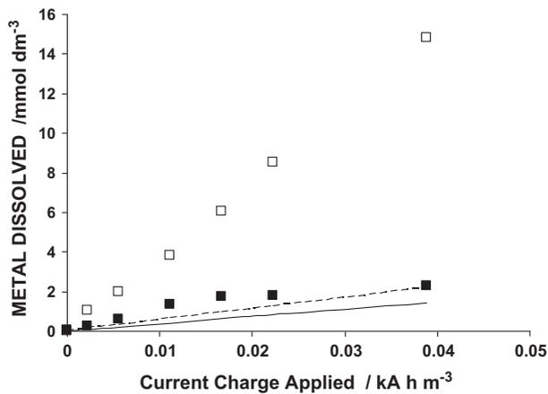
Fig. 2. Variation of aluminium (□) and iron (■) concentration electrogenerated in the electrochemical processes with the electrical charge passed in batch mode operation: Operation conditions:  $T$ : 25°C; flowrate: 50 dm<sup>3</sup> h<sup>-1</sup>; current density: 10 A m<sup>-2</sup>; cell voltage: 3 V. Straight lines: Theoretical values predicted by Faraday's Law.
