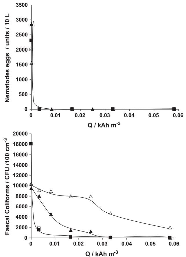
Fig. 7. Variation of the concentration of nematodes eggs and faecal coliforms during the electrocoagulation process of two secondarily treated wastewaters using iron and aluminium electrodes. ▲ WWTP<sub>1</sub>, iron; △ WWTP<sub>1</sub>, aluminium; ■ WWTP<sub>2</sub>, iron; □ WWTP<sub>2</sub>, aluminium. Operation conditions:  $T$ : 25°C; flowrate: 50 dm<sup>3</sup> h<sup>-1</sup>; current density: 10 A m<sup>-2</sup>.
