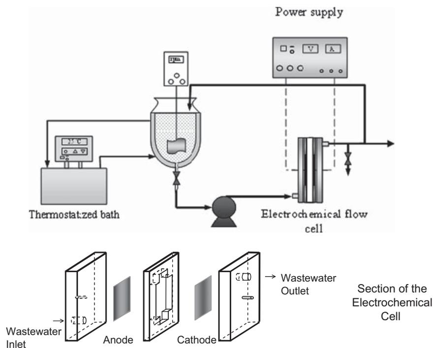
Fig. 1. Layout of the experimental set up and the electrochemical flow cell.
