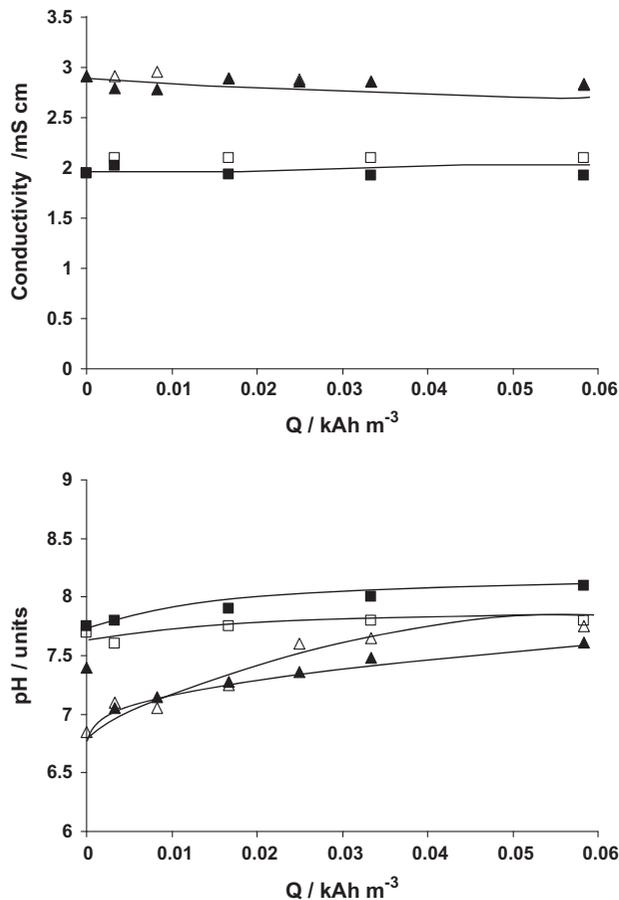
Fig. 6. Changes in the pH and conductivity (after 40  $\mu\text{m}$  filtration) during the electrocoagulation process. WWTP<sub>1</sub> ▲ iron △ aluminium; WWTP<sub>2</sub> ■ iron □ aluminium. Operation conditions:  $T$ : 25°C; flowrate: 50 dm<sup>3</sup> h<sup>-1</sup>; current density: 10 A m<sup>-2</sup>.
