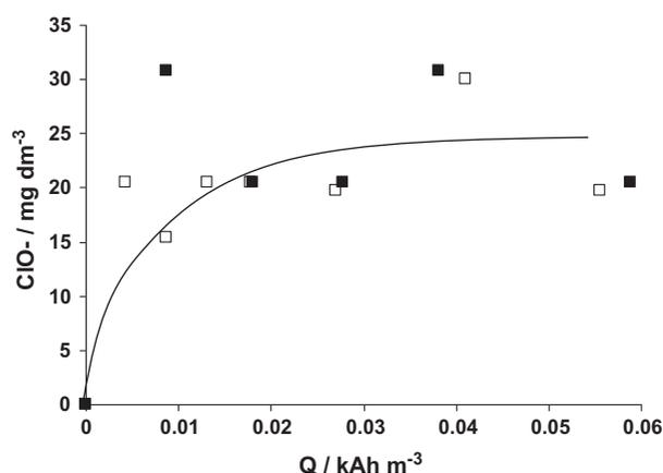
Fig. 8. Production of hypochlorite during the electrolyses of a solution 1.6  $\text{mg dm}^{-3}$  NaCl in the electrocoagulation cells. ■ iron; □ aluminium. Operation conditions:  $T$ : 25°C; flowrate: 50  $\text{dm}^3 \text{h}^{-1}$ ; current density: 10  $\text{A m}^{-2}$ .
