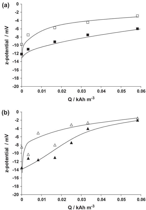
Fig. 4. Changes in the z-potential during the electrocoagulation treatment. (a) WWTP<sub>1</sub> ▲ iron Δ aluminium; (b) WWTP<sub>2</sub> ■ iron □ aluminium. Operation conditions:  $T$ : 25°C; flowrate: 50 dm<sup>3</sup> h<sup>-1</sup>; current density: 10 A m<sup>-2</sup>.
