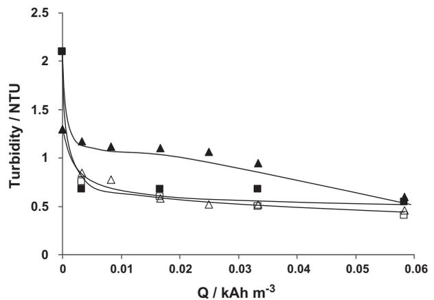
Fig. 3. Influence of the current applied on the removal of COD and turbidity (after 40 μm filtration) WWTP<sub>1</sub> ▲ iron △ aluminium; WWTP<sub>2</sub> ■ iron □ aluminium. Operation conditions:  $T$ : 25°C; flowrate: 50 dm<sup>3</sup> h<sup>-1</sup>; Current density: 10 A m<sup>-2</sup>.
