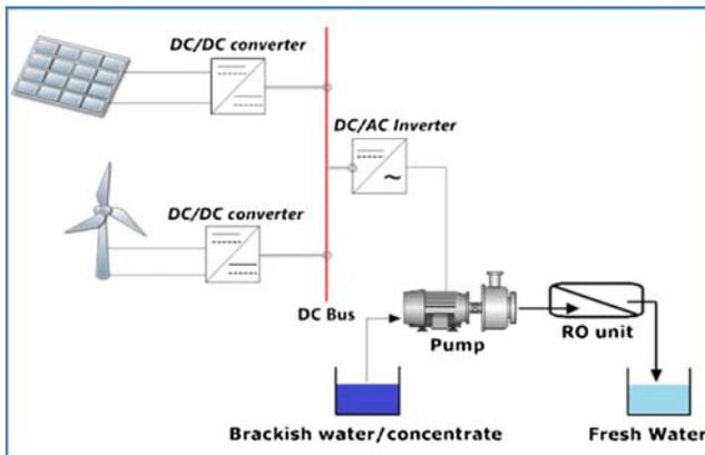
Fig. 1. The configuration of the hybrid PV-wind power plant coupled with a RO desalination unit.
