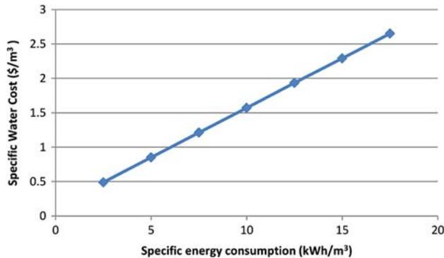
Fig. 8. Linear relationship of the cost of water and specific energy consumption by the RO unit.
