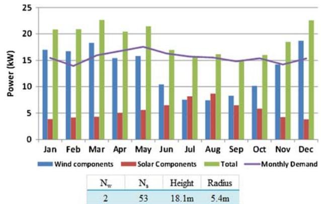
Fig. 5. Monthly power output from the hybrid system components and optimal design parameters.
