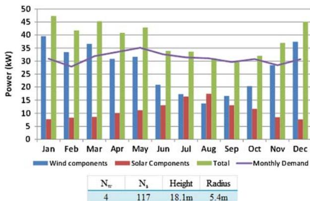
Fig. 6. Output with a specific energy consumption of 5 kWh/m<sup>3</sup> and optimal design parameters.
