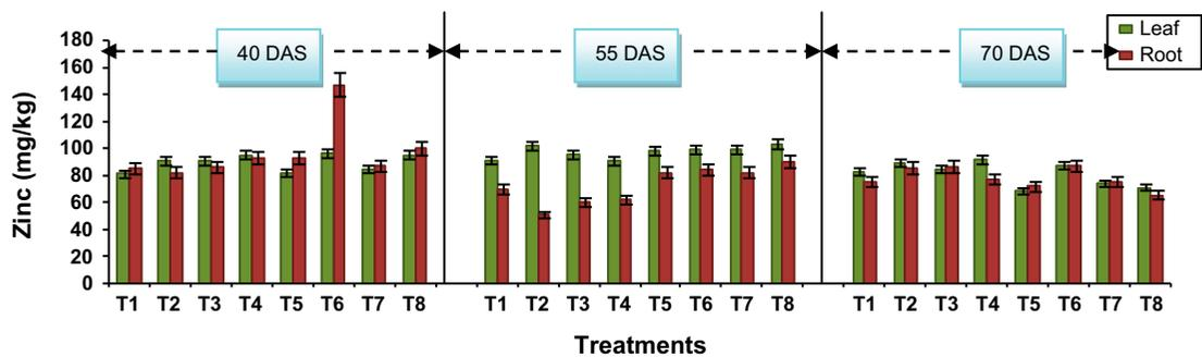
Fig. 13. Zinc concentration in leaf and root at different stages of growth.
