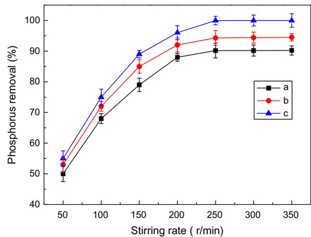
Fig. 8. Effect of stirring rate on the phosphorus removal (a: RM-raw under the adsorption test conditions; b: RM-m under the adsorption test conditions; c: RM-m under the photocatalytic test conditions).
