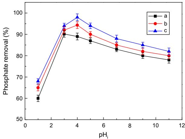
Fig. 5. Effect of initial pH on phosphorus removal (a: RM-raw under the adsorption test conditions; b: RM-m under the adsorption test conditions; c: RM-m under the photocatalytic test conditions).
