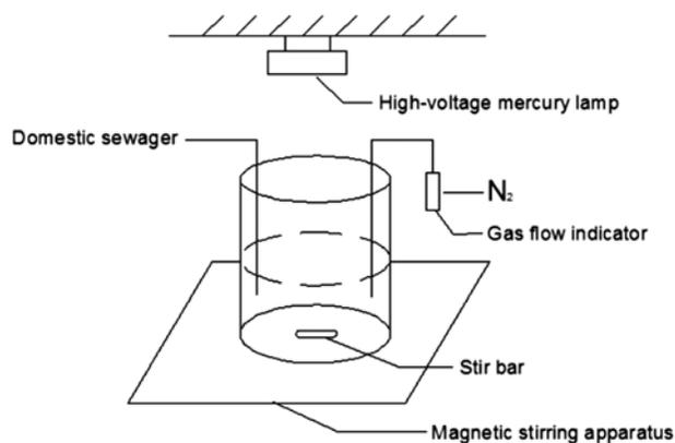
Fig. 1. Sketch of photocatalytic reactor.
