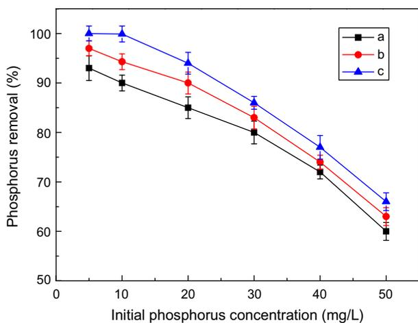
Fig. 9. Effect of initial phosphorus concentration on the phosphorus removal (a: RM-raw under the adsorption test conditions; b: RM-m under the adsorption test conditions; c: RM-m under the photocatalytic test conditions).
