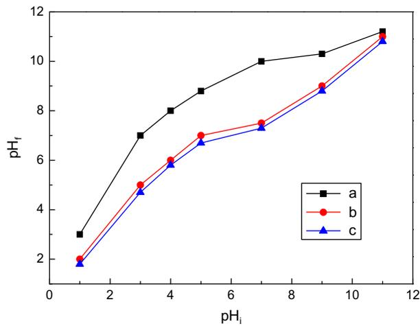
Fig. 6. pH of solution after the reaction (a: RM-raw under the adsorption test conditions; b: RM-m under the adsorption test conditions; c: RM-m under the photocatalytic test conditions).
