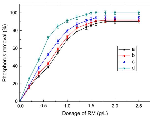
Fig. 4. Effect of RM dosage on the phosphorus removal (a: RM-raw under the adsorption test conditions; b: RM-raw under the photocatalytic test conditions; c: RM-m under the adsorption test conditions; d: RM-m under the photocatalytic test conditions).
