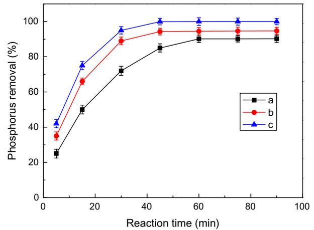
Fig. 7. Effect of reaction time on the phosphorus removal (a: RM-raw under the adsorption test conditions; b: RM-m under the adsorption test conditions; c: RM-m under the photocatalytic test conditions).
