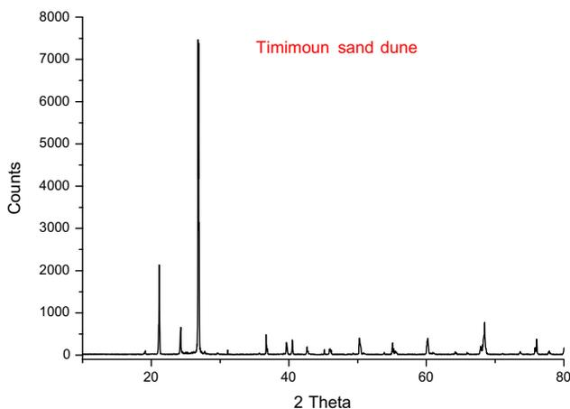
Fig 4. X-ray spectrum of Timimoun sand dune.
