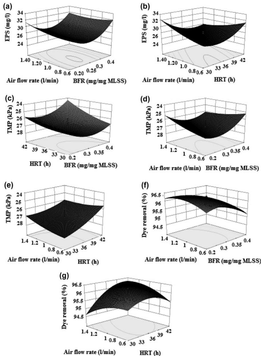
Fig. 4. Response surface for EPS (a)–(b), TMP (c)–(e), and for dye removal (f)–(g).
