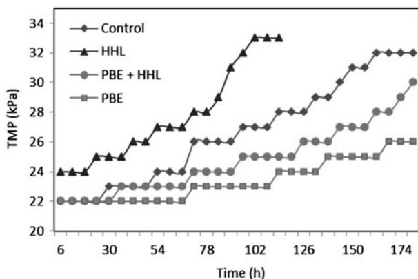
Fig. 5. TMP profiles: verification for biofouling mitigation by QS (PBE: 0.23 mg/mg MLSS, HHL: 1 mg/l).
