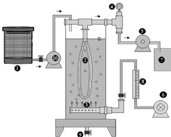
Fig. 1. The reactor setup: (1) feed tank, (2) hollow fiber membrane, (3) air splitter, (4) pressure gauge, (5) peristaltic pump, (6) air compressor, (7) effluent storage tank, (8) air flow meter, (9) drain valve, and (10) feed pump.
