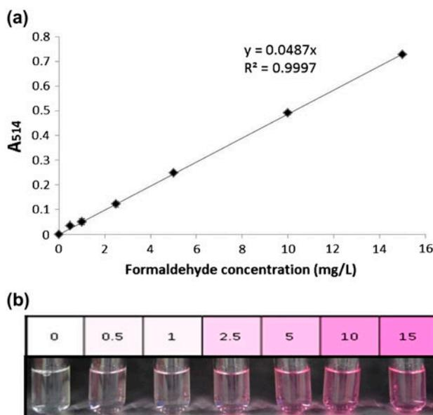
Fig. 4. Standard calibration curve (a) and standard reference colour card (b) for formaldehyde detection using onion juice.
