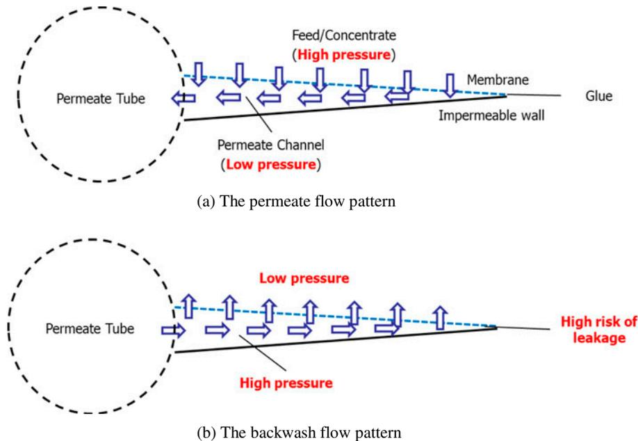
Fig. 1. A cross-sectional view of flow patterns in an unwound membrane leaf of spiral wound RO element.
