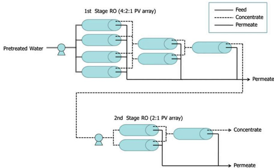
Fig. 2. The flow diagram of the RO pilot plant.
