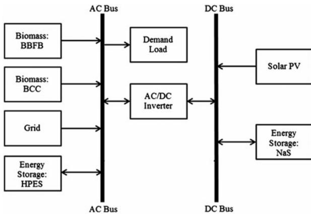
Fig. 2. Configuration of DEG system of UTM.
