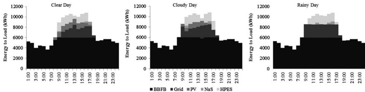
Fig. 5. Energy of various operating units supplied to meet load demands at different weather patterns.
