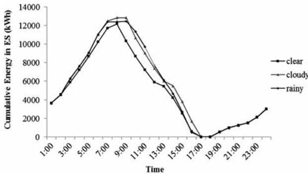
Fig. 7. Cumulative energy in ES at different weather.
