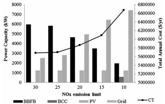
Fig. 8. Impact of reducing NO<sub>x</sub> emission limit on power capacity and total annual cost.
