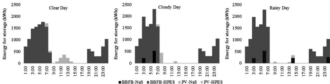
Fig. 6. Energy of various power generators generated for storage in various ES devices.
