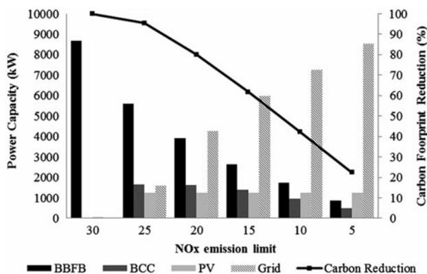
Fig. 10. Impact of reducing NO<sub>x</sub> emission limit on power capacity and carbon footprint reduction.
