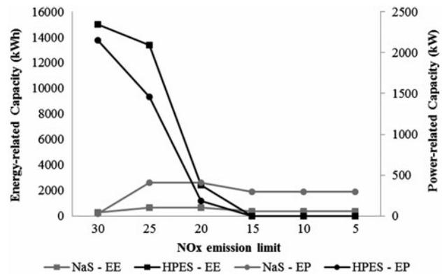
Fig. 11. Impact of reducing NO<sub>x</sub> emission limit on ES capacities (cases of carbon footprint reduction).
