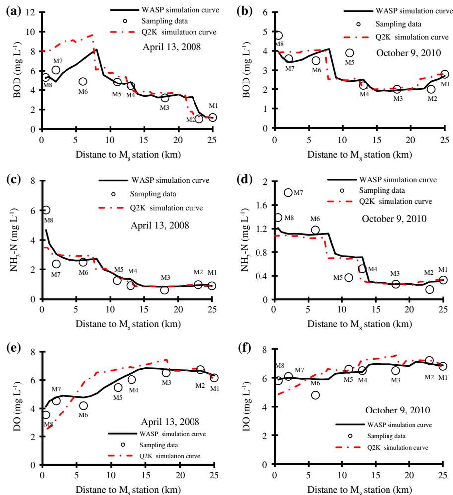
Fig. 3. Water quality model results of CBOD sampled on (a) 13 April 2008 (b) 9 October 2010,  $\text{NH}_3\text{-N}$  on (c) 13 April 2008 (d) 9 October 2010, and DO on (e) 13 April 2008 (f) 9 October 2010.
