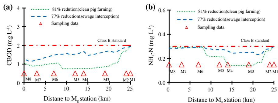
Fig. 6. Variations of (a) CBOD and (b)  $\text{NH}_3\text{-N}$  after implementing the water quality improvement strategies simulated by WASP.
