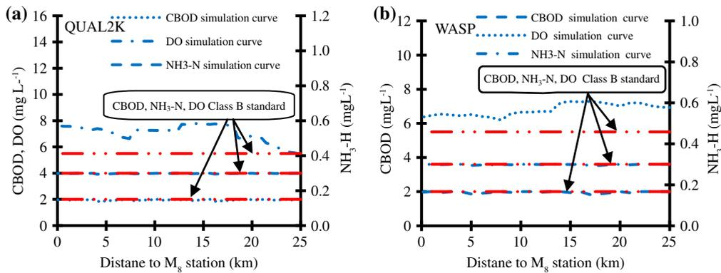
Fig. 4. Simulation results using (a) QUAL2K and (b) WASP model after reducing the pollutant loadings.
