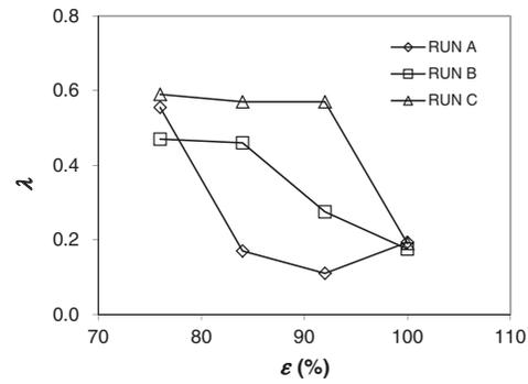
Fig. 7. Effects of porosity on hydraulic efficiencies of FWS CW at various *HLRs*.
