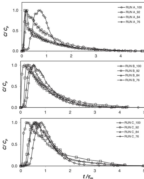
Fig. 5. Comparison of RTDs with porosities 76, 84, 93, and 100% at different *HLRs*.
