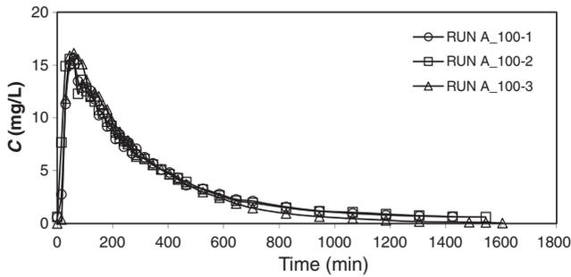
Fig. 2. Sample residence time distribution of fluorescent dye tracer concentration; (RUN A).
