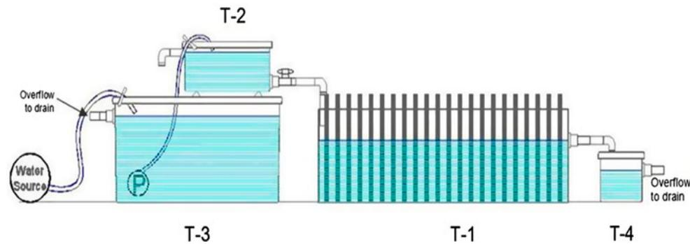
Fig. 1. Laboratory setup for simulating flow patterns induced by artificial vegetation.
