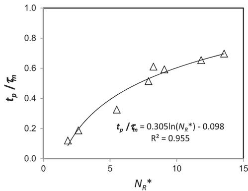
Fig. 8. Relations between the stem Reynolds number and actual hydraulic efficiency.
