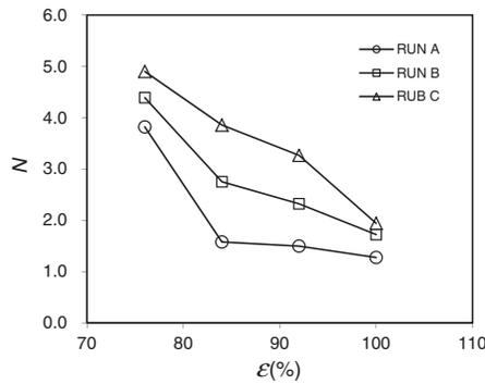
Fig. 6. Variations of number of tanks-in-series affected with different porosity.
