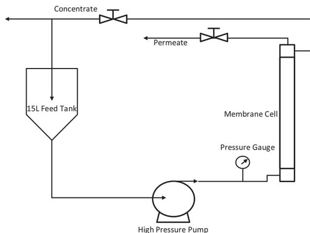
Fig. 2. Laboratory scale filtration unit used to conduct NF and RO experiments.
