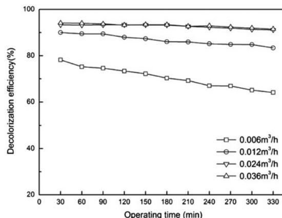
Fig. 4. Effect of aeration intensity on decolorization efficiency of cationic red GTL.
