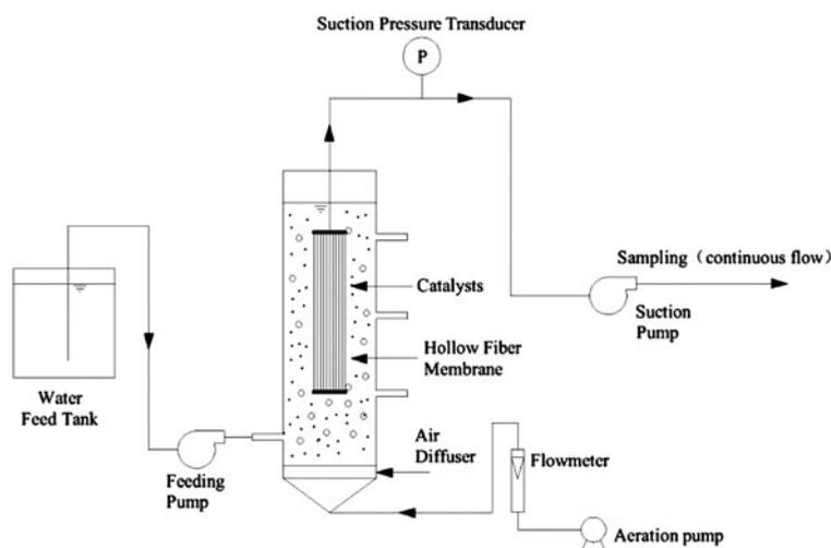
Fig. 1. Schematic diagram of experiment.
