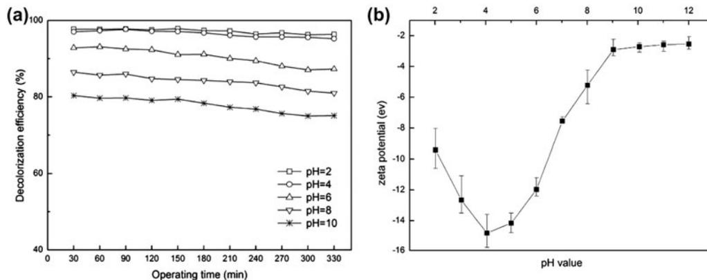
Fig. 6. (a) Effect of pH value on decolorization efficiency of cationic red GTL and (b) zeta potential variation under different pH value.
