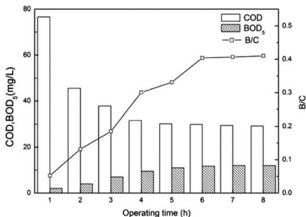
Fig. 9. Biodegradability of membrane effluent in different operating time.
