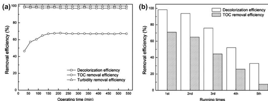
Fig. 7. (a) The color, TOC, and turbidity removal of cationic red GTL dye using hybrid system in continuous mode and (b) the color and TOC removal in the single CWAO batch test.
