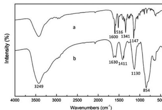
Fig. 8. FT-IR spectra of cationic red GTL (a: original wastewater b: effluent of membrane).
