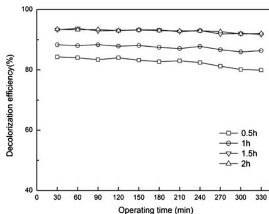
Fig. 2. Effect of residence time on decolorization efficiency of cationic red GTL.
