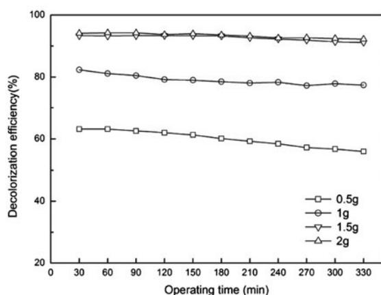
Fig. 3. Effect of Mo/Zn/Al/O catalyst dosage on decolorization efficiency of cationic red GTL.
