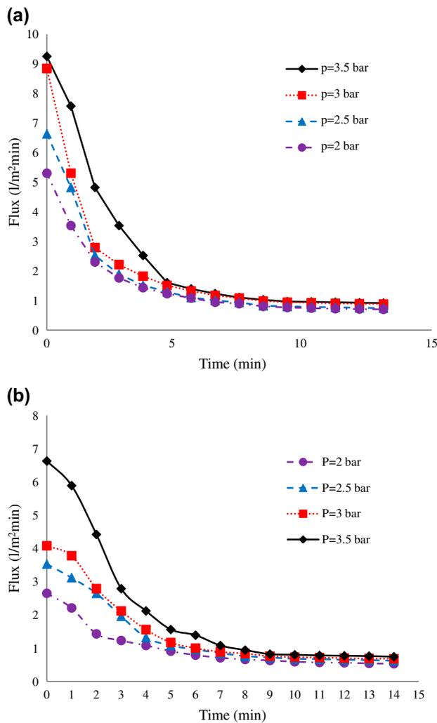
Fig. 3. Time variation of flux at different TMPs using: (a) CPC and (b) CTAB.
