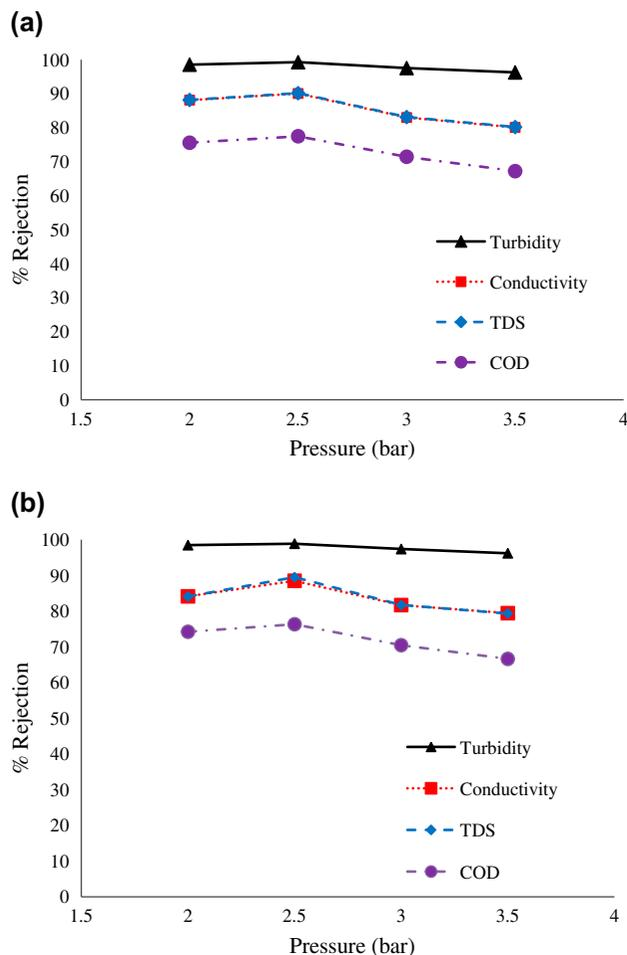
Fig. 6. Effect of TMP on rejection percent of pollution indicators using: (a) CPC and (b) CTAB.
