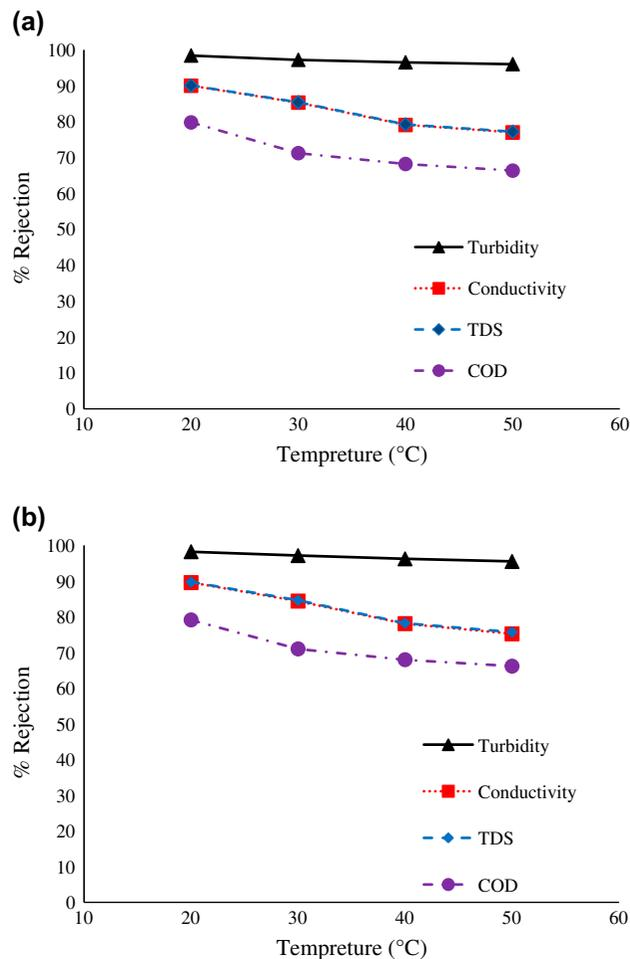
Fig. 7. Effect of temperature on rejection percent of pollution indicators using: (a) CPC and (b) CTAB.
