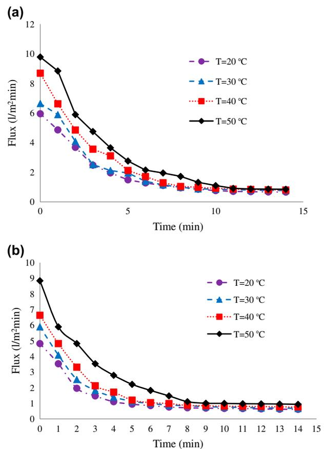
Fig. 4. Time variation of flux at different temperatures using: (a) CPC and (b) CTAB.
