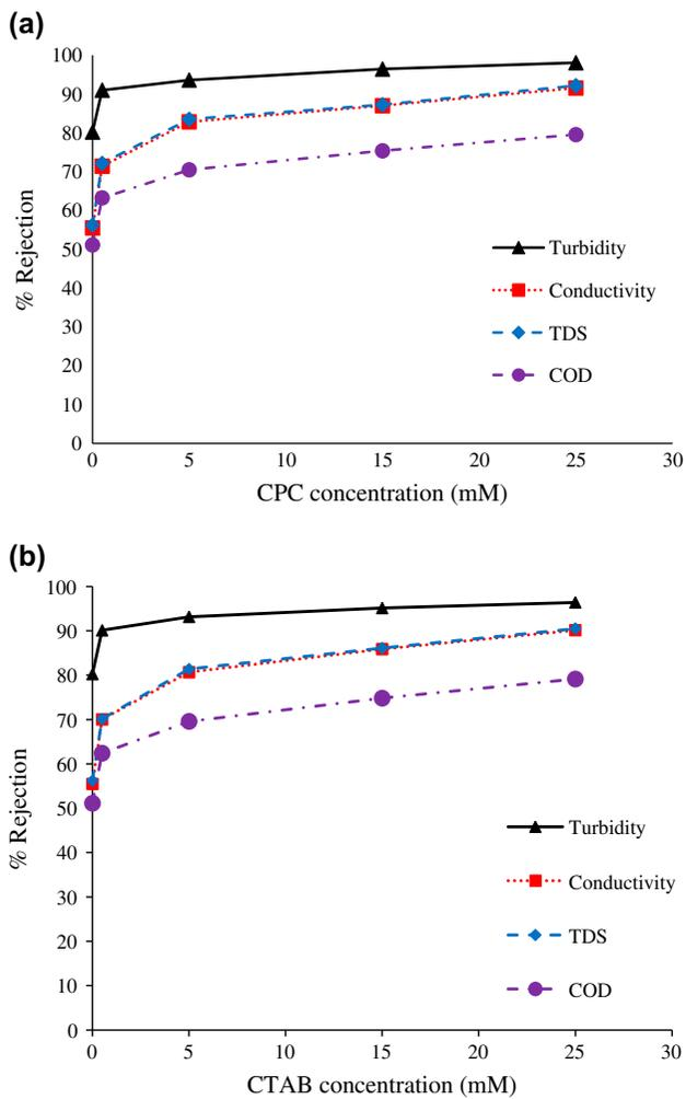
Fig. 8. Effect of surfactant concentration on rejection percent of pollution indicators: (a) CPC and (b) CTAB.
