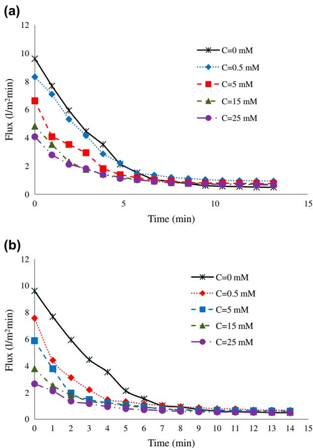
Fig. 5. Time variation of flux at different surfactant concentrations: (a) CPC and (b) CTAB.
