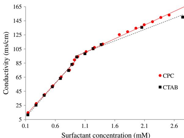
Fig. 2. Determination of CMC for CPC and CTAB through conductivity measurement.
