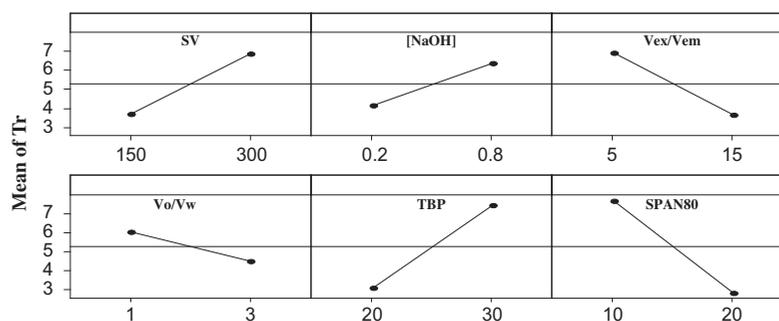
Fig. 2. Main effects plot (data means) for  $T_r$ .
