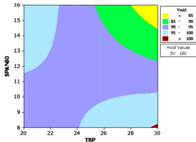
Fig. 10. Contour plot of yield vs. SPAN80; TBP.
