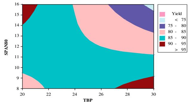
Fig. 5. Contour plot of yield vs. SPAN 80; TBP.
