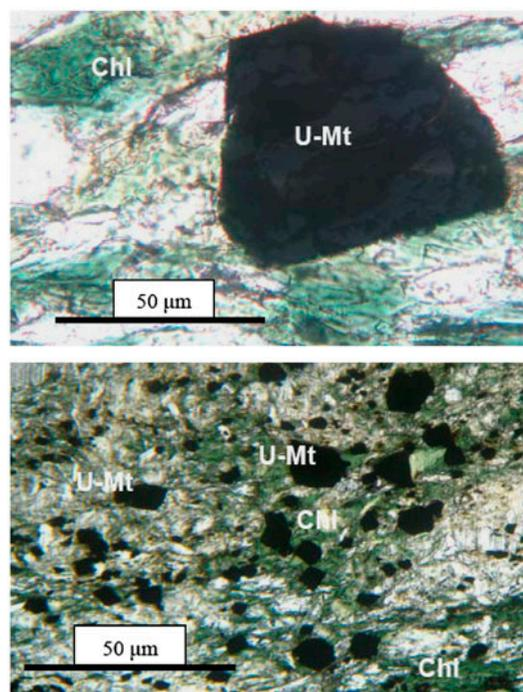
Fig. 2. Microstructure of Narwapahar ore shows uraninite–magnetite (U-Mt) grains distributed within chlorite–quartzofeldspathic.
