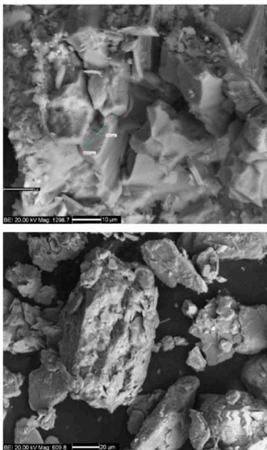
Fig. 10. Scanning electron micrograph of ore particles before and after acoustic leaching.
