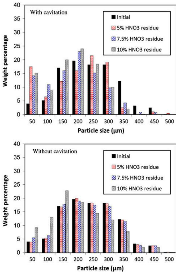
Fig. 7. Particle disintegration of MgF<sub>2</sub> with and without cavitation.
