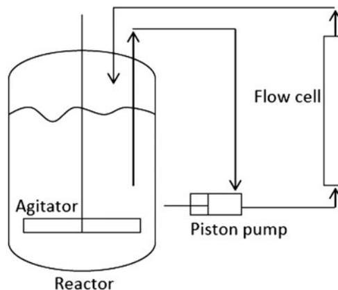
Fig. 3. Experimental set up for ore leaching with acoustic cavitation by flow cell.
