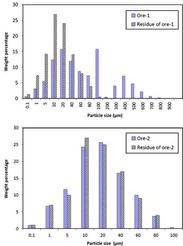
Fig. 9. Ore particle disintegration during acoustic leaching.
