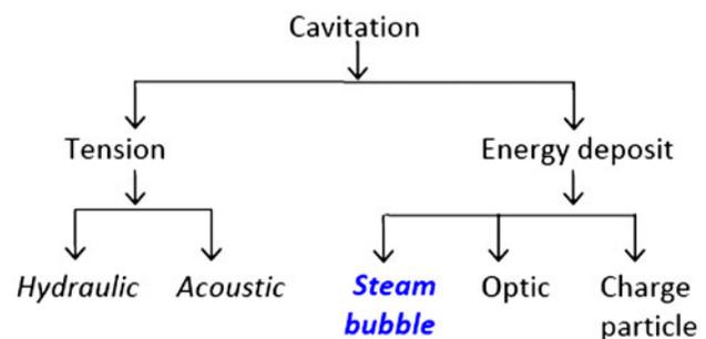
Fig. 1. Different techniques of cavitation.
