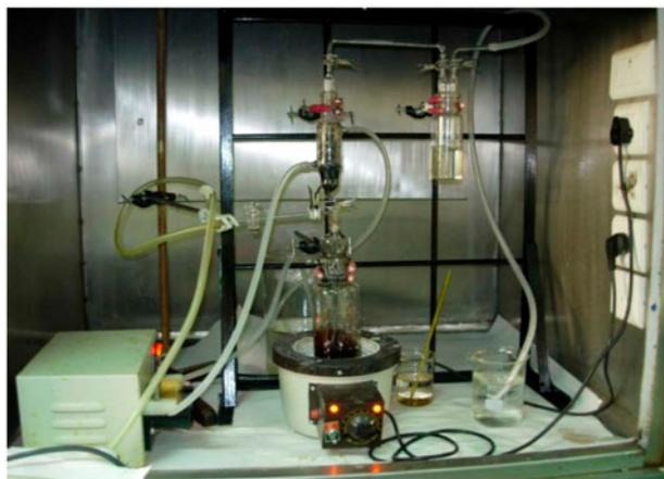
Fig. 1. Experimental set-up for volatilisation cum adsorption. Ru concentration 126–500 ppm, nitric acid concentration 2–6 M, temperature 60–80°C, adsorbent PEEK, silicone tubes, oxidant KMnO<sub>4</sub>, O<sub>3</sub>, K<sub>2</sub>S<sub>2</sub>O<sub>8</sub>.
