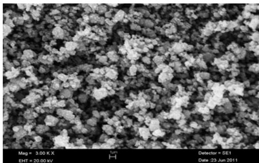
Fig. 3. SEM image of potassium zinc ferrocyanide powder.
