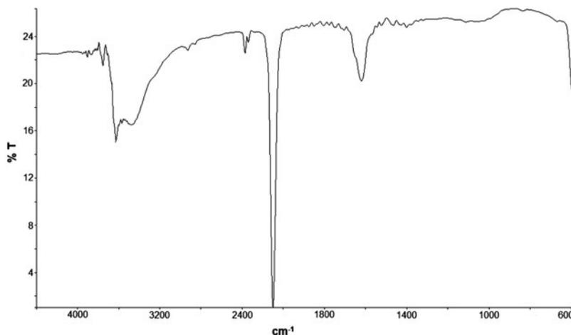
Fig. 1. FT-IR of potassium zinc ferrocyanide powder.
