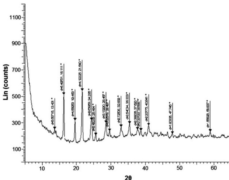
Fig. 2. XRD of potassium zinc ferrocyanide powder.
